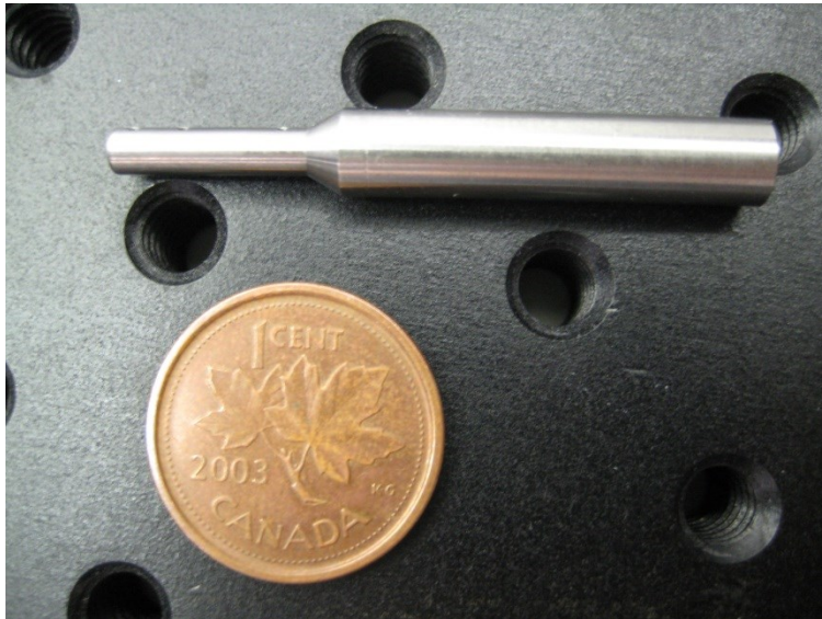
Figure 37: Photograph of the barrel housing the focusing optics
