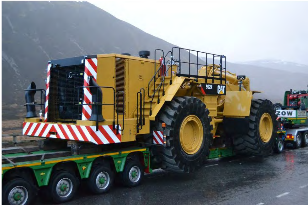
Photo 2.3: Demobilised CAT 992K Loader in Transit
