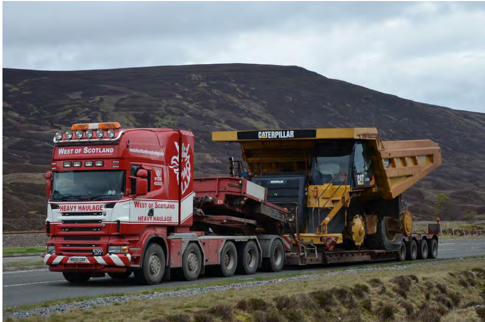
Photo 2.1: Demobilised CAT 777F Dumper Truck in transit
