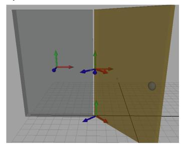
This example demonstrates a door with a hinge. The wall rigid body (in gray, on the right) has its local space frame in its center. The door has its local space on the floor and rotated 45 degrees on the y axis. The hinge constraint is limited to rotate +/- 90 degrees on its y axis. Each attachment frame has its translate/rotate transforms defined in terms of the rigid body's local space.
