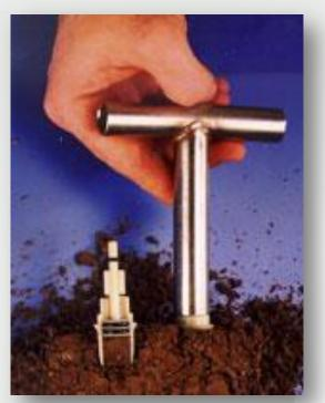
En Core ® Sampler and sampling handle
