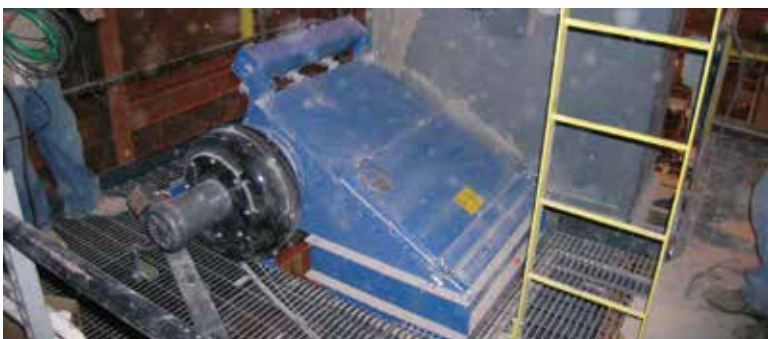
CPV - Bucket Elevator 1,200 cfm (2,038 m 3 /h)
