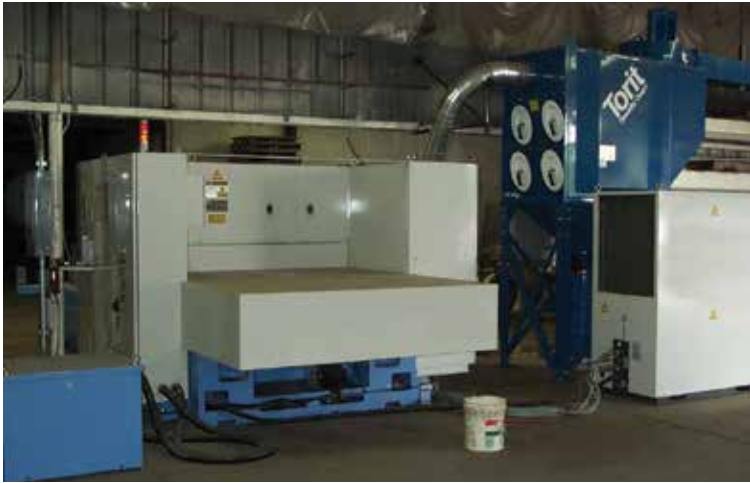
DFO on Laser Cutting 3,100 cfm (5,266 m 3 /h)
