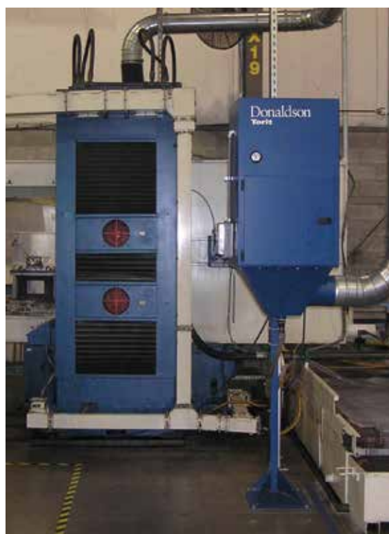
WSO - Horizontal Grinder 850 cfm (1,444 m 3 /h)
