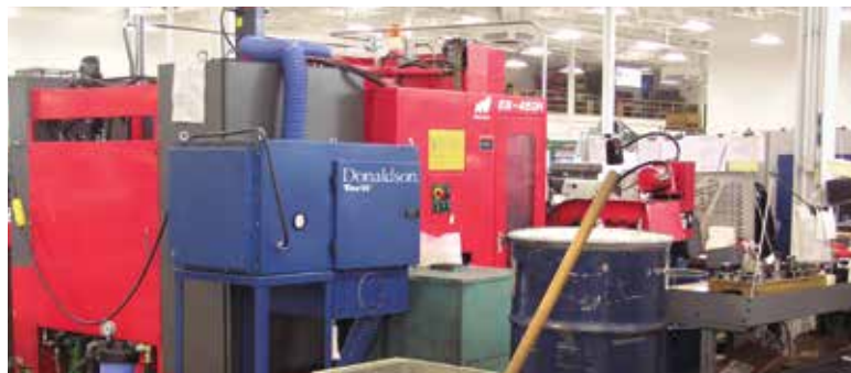
DMC on Machining 800 cfm (1,359 m 3 /h)
