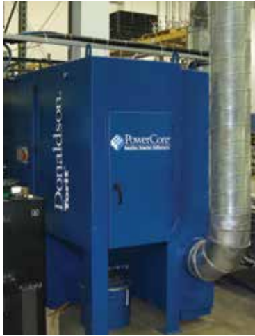
TG on Plasma Cutting 2,300 cfm (3,90 m 3 /h)
