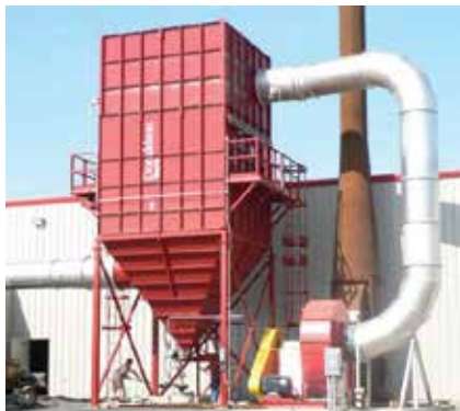
MB on Glass Processing 25,000 cfm (42,466 m 3 /h)
