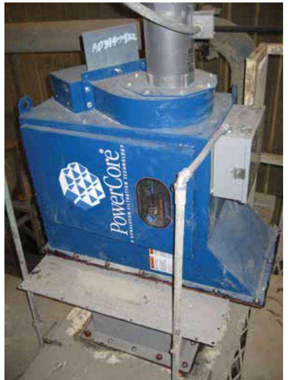
CPV - Feed Hopper 350 cfm (595 m 3 /h)
