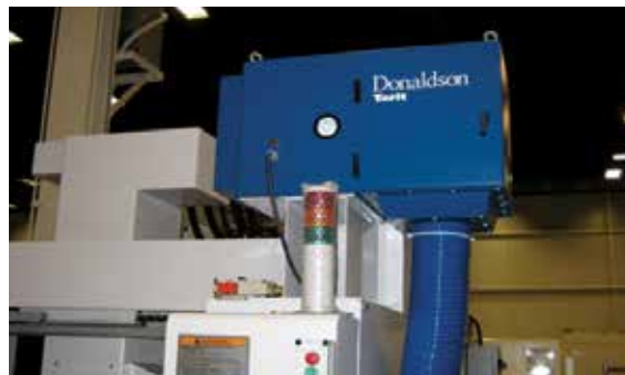
DMC on Wet Machining 390 cfm (662 m 3 /h)
