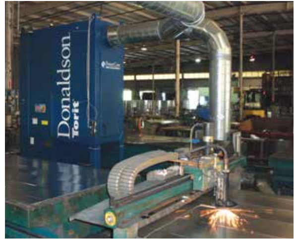
TG on Plasma Cutting 3,400 cfm (5,775 m 3 /h)
