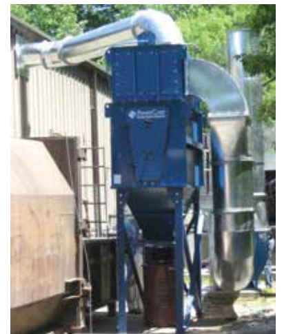
VH on Grinding 9,000 cfm (15,288 m 3 /h)
