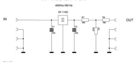
When comparing this circuitry to the TS-830S circuitry in the narrow CW slot, it seemed like a very favorable substitute for the YC-455C. The input/output impedance for the YG-455C is 2k ohm shunted by approx 15pf.
