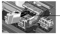
Do not touch the lock lever; remove only the ink tank.
