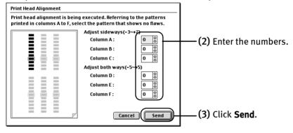
Note If this is difficult to pick up the best pattern on Column F, pick the setting that procedures the least noticeable vertical white stripes.
