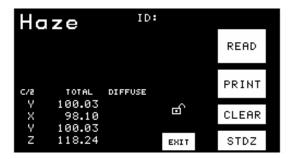
You are prompted to read the sample with black at the reflectance port. Leave your sample at the transmission port and then mount the light trap at the reflectance port.
