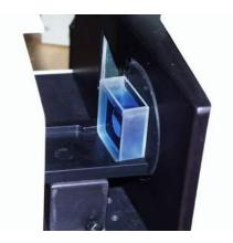
The transmission cell holder holding a 20-mm cell at the sphere opening.
