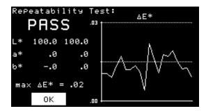
If the max  $\Delta E^*$  shown at the bottom of the screen is less than or equal to **0.03** for measurements of the white tile or **0.05** for measurements of air, your instrument passes the test. Touch **OK** to exit this screen.
