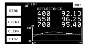
On the measurement screen, you may touch the **Stdz** button to initiate instrument standardization as described earlier in this chapter. Touch the **Print** key if you are using the optional printer and wish to print the measurements as currently displayed. You may also touch the **Clear** key once to clear the sample reading and then again to clear the standard reading, if there is one. Touching **Exit** returns you to the Select an Applet screen.
