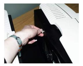
6. Remove the front cover from the instrument by sliding it forward and unplug the harness which connects the indicator lights of the front cover to the instrument.
