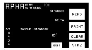
To initiate a reading, either touch the **Read** button on the touch screen or press the Macro/Read button on the body of the ColorQuest XE. The sample will be read and its absolute tristimulus values and index data displayed.
