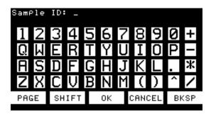
Type in the desired ID and then touch **OK** to apply it. IDs may consist of up to fourteen alphanumeric characters unless you are using a custom applet that has defined a different number of characters. You may touch the **Page** button to move to a second page of available characters.
