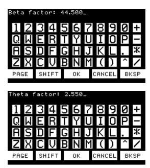
When you touch **OK** after entering the Theta factor, the measurement screen then shows Saybolt\*, indicating that the Saybolt factors have been optimized. Measure Saybolt as you ordinarily would.
