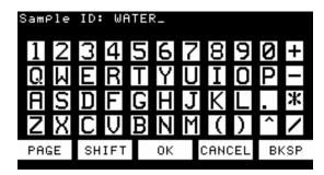
14. Type an ID on the keypad. In our example, "Water" was chosen. When you finish typing, touch **OK** to accept the ID. The ID is then shown at the top of the screen. If you make a mistake, touch **Bksp** to back up and fix it.
