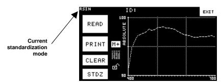
If you wish this measurement to be stored as the standard, touch the M+ button to store it. The M+ button changes to an M indicating that a standard has been stored. This standard will be available whenever this applet is used until you clear it using the **Clear** button.
