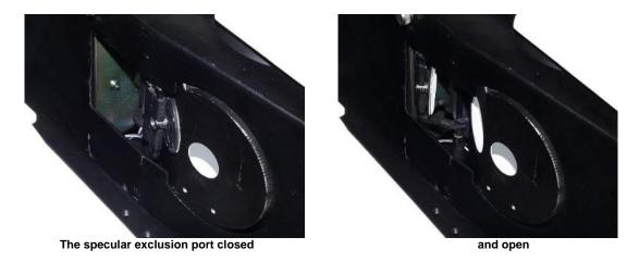
The ColorQuest XE features automated specular included/excluded port control and sensing. This feature allows you to set the port to the desired position from the touch screen. The screen reports the position, thereby allowing errorless measurements.
