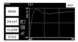
11. Touch any area on the reflectance plot. The wavelength you chose and the standard, sample, and delta values for that wavelength will appear above the plot.
