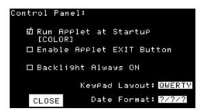
If you wish for users to be able to use the **Exit** button to leave applets even when they are locked, touch the box next "Enable Applet EXIT Button" so that it is checked.
