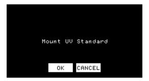
5. Place the fluorescent standard at the reflectance port, centering spot 3 at the port. Use the dotted guides on the labeled side of the standard to properly center the standard under the sample clamp. Touch **OK** and then the following screen appears.
