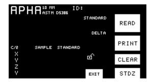
3. Touch APHA, multiple times if required, until 20 mm ASTM D5386 is shown next to it.
