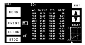
In the 3 Points applet, you may touch any of the three displayed wavelengths to increase its value by 10 nm.
