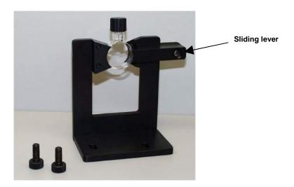
To install the holder, position it so that the holes in its base are down toward the floor of the transmission compartment and the cutout in the vertical section is at the transmission port (hole in the sphere). The base holes should be positioned over two of the threaded holes in the transmission compartment floor. Insert the two thumbscrews provided and tighten.
