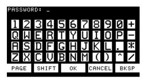
To assign an ID to the last measurement, touch the ID area at the top right of the screen. A keypad will appear on the screen.
