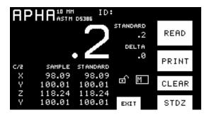
Touch the **Read** button on the touch screen again or press the Macro/Read button on the body of the ColorQuest XE to read a sample. The sample will be read and its absolute tristimulus values and index data displayed. The value for the main index of interest (APHA in this example) will also be shown in large numerals at the top of the screen.
