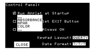
Touch the name of the applet you wish to run at startup. It is then shown underneath the checked box.
