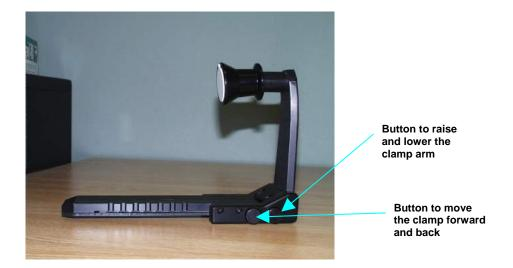
A magnetic white ceramic disk on the face of the clamp provides a consistent white background for measurements. A non-slip black pad (also magnetic) is also included that can be used to replace the white disk for applications that require a non-slip or dark backing. To change to the pad, simply pop out the white disk and insert the non-slip pad.
