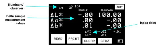
On the measurement screen, you may touch the **Stdz** button to initiate instrument standardization as described earlier in this chapter. Touch the **Print** key if you are using the optional printer and wish to print the measurements as currently displayed. You may also touch the **Clear** key once to clear the sample reading and then again to clear the standard reading. Touching **Exit** returns you to the Select an Applet screen.
