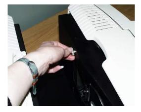
6. Remove the front cover from the instrument by sliding it forward and unplug the harness which connects the indicator lights on the front cover to the instrument.
