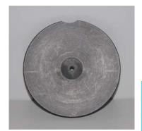
This option provides a modified port plate with a 4-mm round opening. This port plate should only be used when the small area view option is available and in use. To install the port plate, remove the standard port plate and snap the modified port plate into place at the reflectance port. Standardize the instrument in a reflectance mode using small area view.
