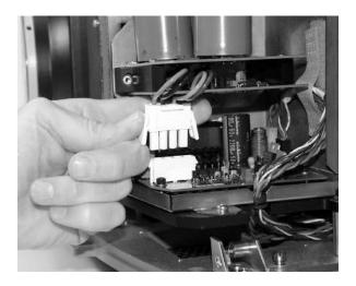
9. Remove the lamp assembly and replace with a new assembly. Be sure not to touch the bulb of the lamp, as fingerprints reduce lamp efficiency and weaken the glass. If a fingerprint is deposited, remove it using a clean wipe and isopropyl alcohol.
