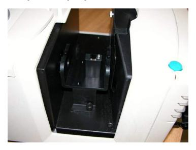
4. When prompted for the cell blank, fill the desired analytical cell with distilled water or another clear liquid you would like to use as your top of scale. Some cells will have a fill line. The liquid should at least reach this line.
