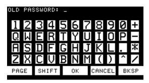
First, enter the old password and then touch **OK**. If your system is brand new, type HUNTERLAB and touch **OK**, since that is the default system password.
