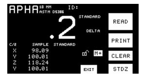
If you wish this measurement to be stored as the standard, touch the **M**+ button to store it. The **M**+ button changes to an "M" indicating that a standard has been stored and the measurement values move to the standard column. This standard will be available whenever this applet is used until you clear it using the **Clear** button.
