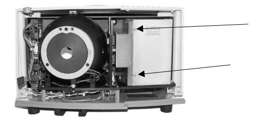
8. Unplug the white connector of the lamp assembly by squeezing the latches on the sides of the connector.
