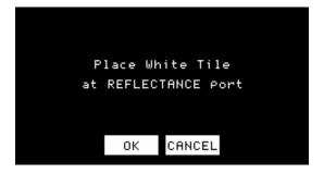
10. Mount the white tile at the reflectance port as instructed and either touch **OK** or press the Macro/Read button on the instrument. The ColorQuest XE reads and then returns you to your measurement screen. Standardization is complete.
