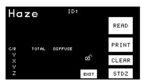
First, standardize the instrument in TTRAN mode by touching **Stdz** and following the on-screen prompts. In the haze applet only, a third prompt is added to the standardization process as shown below. It requires you to mount the light trap at the reflectance port.
