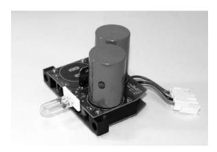
Before you attempt to change the source lamp, ensure that the UV filter is out. If the UV filter is left in, the filter may be broken during the process of removing and re-inserting the bezel. Check the UV Excluded indicator light. If the indicator light is on, you must restandardize the sensor in a mode with the UV filter out. (The filter can also be manually removed from the path, if necessary, by a trained representative of HunterLab.)
