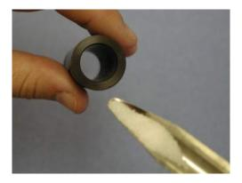
4. Pack the powder down using the plunger. Do not overtighten the powder holder. The powder should be at least 1/2-cm deep in the holder.
