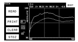
Press the miniature table icon to show the actual reflectance or transmittance values. To go back to the plot screen, press the miniature plot at the bottom right of this screen. Use the **up and down arrow** buttons to scroll upward and downward through the data.
