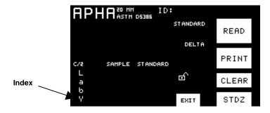
6. Touch the index area (which says "Y" in the screen shown above) until YI is shown. You may be required to touch and release the index multiple times before YI is displayed.
