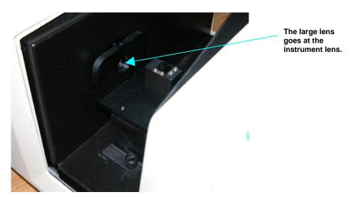
2. Ensure that the holder is in a straight line between the instrument lens and the hole in the sphere. Depress and turn the captive thumbscrews clockwise into holes in the transmission compartment floor. If the holder is slightly off-line, reposition it so that the screws align properly with the holes on the floor of the transmission compartment.
