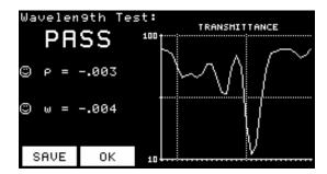
$\rho$  indicates the photometric error since the test values were last stored.  $\omega$  is the wavelength misalignment since the test values were last stored. If  $\rho$  is greater than **0.1** or  $\omega$  is greater than **1.0**, the instrument fails the test and you should check the following:
