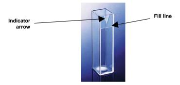
5. Slide the transmission cell into the cell holder as far as it will go. If your cell has an indicator arrow, point it toward the hole in the instrument sphere.
