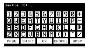
12. Type an ID on the keypad. In our example, "Water" was chosen. When you finish typing, touch **OK** to accept the ID. The ID is then shown at the top of the screen. If you make a mistake, touch **Bksp** to back up and fix it.
