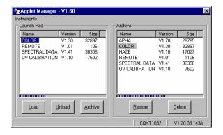
The <u>Launch Pad</u> side of the screen indicates those applets currently in your instrument's loaded memory. The <u>Archive</u> side shows the applets available in your instrument's archives. The status bar at the bottom of the screen indicates your sensor serial number and firmware version.
