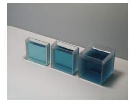
For transmission measurements, use the cell size recommended by your measurement specification (such as an ASTM method),
