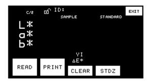
To initiate a reading, either touch the **Read** button on the touch screen or press the Macro/Read button on the body of the ColorQuest XE. The sample will be read and its absolute tristimulus values displayed.
