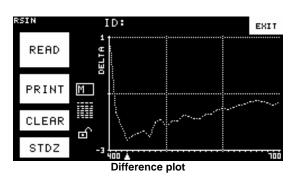
Touch any wavelength on the plot to show the sample, standard, and delta reflectance or transmittance for that wavelength. "S" indicates the sample, "M" indicates the standard, and "D" indicates the delta, or difference, data.
