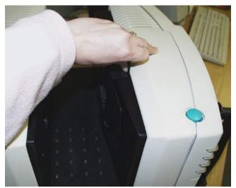
Standardizing on the black card device for TTRAN mode. (The transmission compartment door may be closed down to the device handle.)
