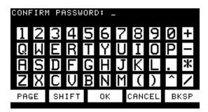
Enter the new password a second time and touch **OK**. The password is then changed from the old to the new.
