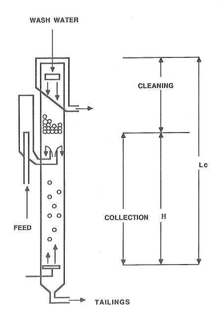
FIGURE 1 Flotation Column.
