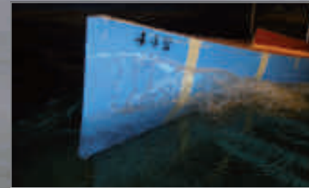
TESTING THE AXE BOW HULL FORM
