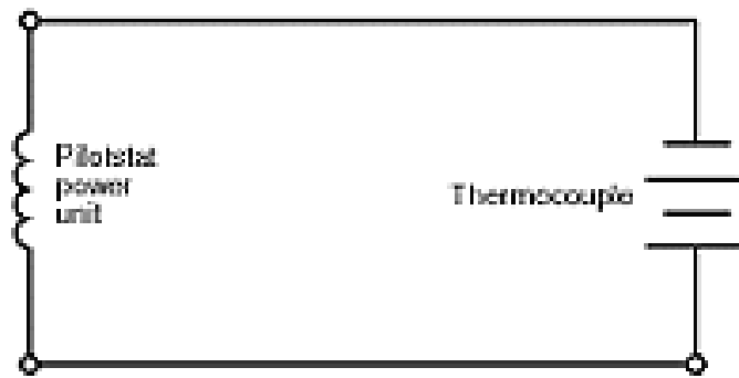
FIGURE 11 — Safety Shutoff Circuit.
