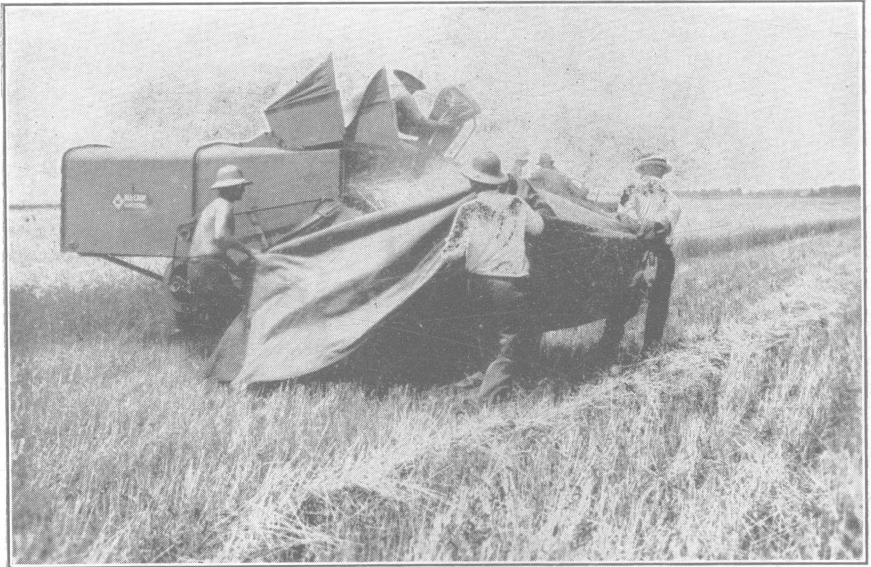
Fig. 2.—Collecting straw and chaff during a test
