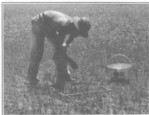
Fig. 4.—Collecting cutter bar losses
