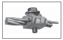
Interlocking finger design accommodates large range of conductor sizes. Tin-plated, cast of high copper alloy and clamped with plated steel bolt, PENETROX<sup>TM</sup> joint compound recommended with aluminum and ACSR.
