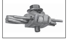
Interlocking finger design accommodates large range of conductor sizes. Tin-plated, cast of high copper alloy and clamped with silicon bronze DURIUM™ bolt, PENETROX™ joint compound recommended with ACSR. Applications include grounding for the Cable TV industry.
