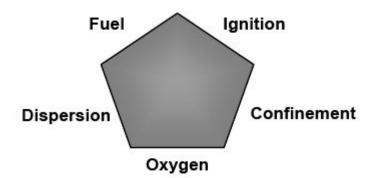
The combustible dust is the fuel. The dispersion is any event that causes settled dust to become airborne. The confinement could be the process equipment, ductwork, a storage vessel, or silo. The ignition source could be static electricity or anything that causes a spark. The suspended dust if ignited burns rapidly, and confinement allows for rapid buildup of pressure resulting in an explosion.
