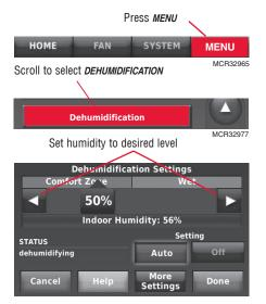
This feature can control your air conditioner to reduce humidity. Move the slider bar to the humidity level you prefer, then press **DONE**.
