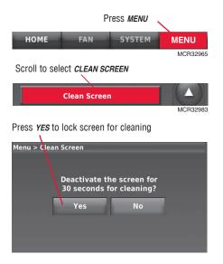
Use this feature to lock the screen so you can clean it without changing any settings. A countdown timer will show elapsed time until the screen is reactivated.
