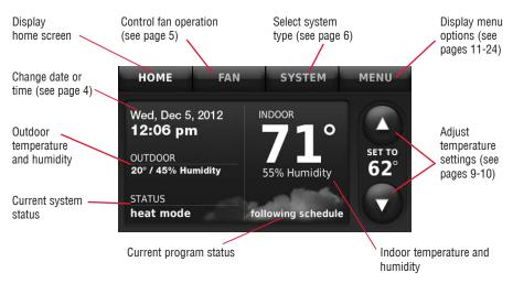
Outdoor temperature and humidity are displayed only if an optional outdoor air sensor is installed.
