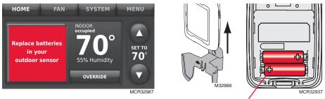
Remove sensor from bracket, detach cover and install 2 fresh AA lithium batteries
