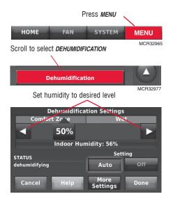
Move the slider bar to the humidity level you prefer, then press **DONE**. If your air conditioner is used to control humidity, the thermostat may use the following methods to maintain your desired humidity:
