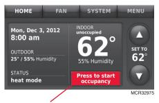
Press to maintain comfortable temperature while room is occupied
