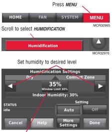
Window Prótection limits the amount of humidity to prevent frost or condensation on windows 69-2687EFS—01 Move the slider bar to the humidity level you prefer, then press *DONE*.
