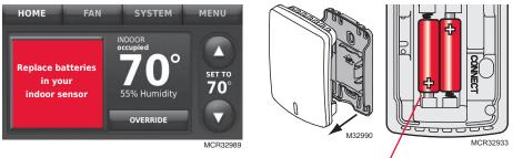
Install 2 fresh AAA alkaline batteries. Status light will briefly flash green. If it flashes red, batteries are not good.
