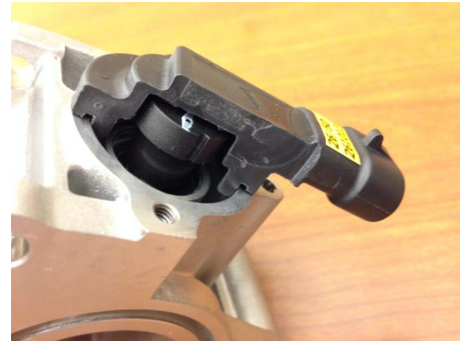
Section view of Contactless TPS
