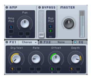
The signal flow in the Output Sections passes first through the Amp Section, including the Pan Control, then through Master Effect 1, then Master Effect 2, and then finally out through the Master Volume knob. Note that the parallel voices are combined to a stereo down-mix after the panorama section and before the master effects. See section \$\frac{1}{3}.1\$, Signal Flow and Voicing for more information.
