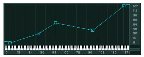
When you click on a Breakpoint, both the x- and y-axis display small lines pointing to their coordinates. The coordinate numerical values are also displayed in the two small fields at the right of the horizontal axis and at the bottom of the vertical axis. If you double-click on a particular Breakpoint, you will delete the whole User Response and replace it by a horizontal line at the Breakpoint's vertical level, thus creating a constant key-tracking response at this particular outgoing pitch.
