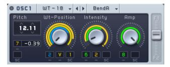
The range of influence of the Macro Control over the control it is affecting is proportional to the corresponding yellow ring around the control. For example, in the image above we can see that the influence of Macro Control 2 on the Intensity knob is greater than that of the green modulation source indicated by the numeral "6". The different color reflects that this modulation source is not a Macro Control, but an LFO. The blue "2", finally, denotes an envelope generator.
