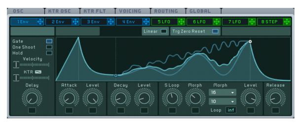
The Center Window display can be switched between eight **modulation sources** and six pages of **general settings**. You can choose which page of controls to access by clicking one of the two rows of labeled tabs across the top of the Center Window. Please note that these tabs are not hierarchical in any way, i.e. all of the tabs for both the modulation sources and the general settings are visible at all times regardless of which tab is active in the upper row.
