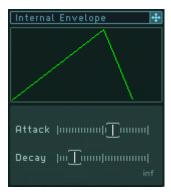
In the lower part of this block, you will find two parameters to control this envelope: the *Attack Time Fader* adjusts the attack of the envelope, and the *Decay Time Fader* adjusts its decay. All adjustments are represented on the *Internal Envelope Graphic Display*.
