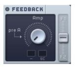
In the Feedback Section, you can adjust the level of output using the Amp level knob, and adjust the ratio of the output between filter 1 and filter 2 using the Routing Fader. The Amp knob has 2 modulation slots where you can attach a modulation source to change the output.
