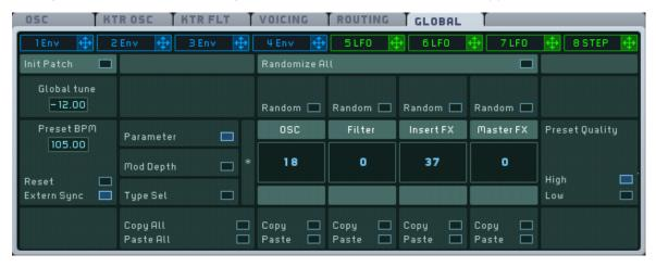
The eight **modulation sources** are grouped into envelopes (slots 1-4) and assignable pages (slots 5-8) that allow you to choose between the *LFO*, *Performer*, and *Stepper* modulation sources. If you have chosen one of these assignable slots, you can choose one of these types by using the popup menu in the upper-right corner of the modulation source page.
