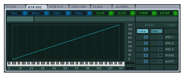
The Keytracking Oscillator Page is divided into two parts: at the left, a *Mapping Area* shows how the current keytracking response is set up; on the right, a *Mapping Selector* allows you to map this keytracking response to the individual oscillators.
