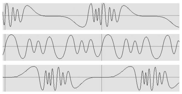
BendA mode only uses the two upper settings, i.e. the Intensity knob only morphs between the upper image (controller at the left) and the middle image (controller at the right). The third bend mode, finally, only interpolates between the middle image (Intensity at the left) and the lower image (Intensity at the right).
