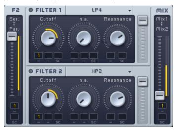
Note that there is also a Mix Control at the right side of the filter section. It controls which filter's signal is used as the filter section's output. You can blend between the first filter's signal (at the top) and the second filter's signal (at the bottom); in between, both signals are mixed.
