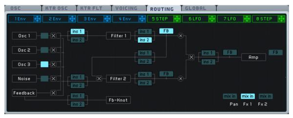
As you can see in this picture, there are a number of small buttons labeled "ins1" and "ins2" present in the Routing Page, placed in various positions between the oscillators, filters and other components of MASSIVE. These buttons are the *Insert Effects Position Selectors*. You can use these to select where exactly each Insert Effect should be placed to modify the sound. Simply click one of the buttons labeled "ins1" to select where the Insert 1 effect will be placed, for example.
