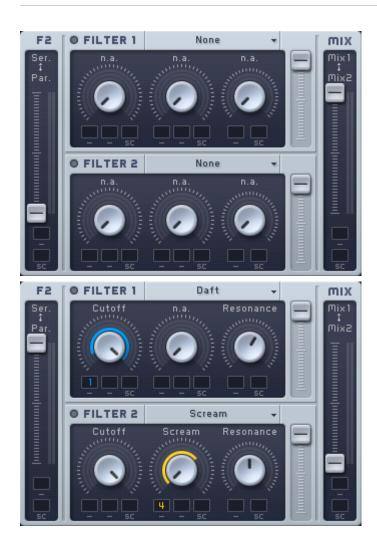
First, set the *Filter Input Fader* (labeled *F2* and marked "Ser<>Par") all the way to the top. This sets up a **serial** filter routing, such that the second filter takes the first filter's output signal as its input signal. In this example, we want the two filters to process the signal subsequently one after another, not parallel/simultaneously.
