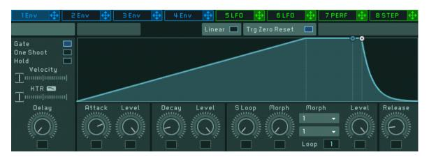
This page shows us the controls of one of MASSIVE's four **envelope generators**. Envelopes are signals that first rise when a note is played, stay at some fixed level as long as the key is held (usually), and then fall back to zero when the note is released. Envelopes are often used to define the volume of a note, becoming louder when a key is pressed, holding that volume, and decaying when the note is released.
