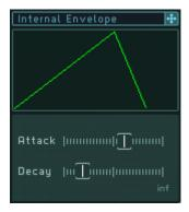
In the lower part, you will find two parameters for this envelope: the *Attack Time Fader* adjusts the attack of the envelope, and the *c* adjusts its decay. All adjustments are represented on the *Internal Envelope Graphic Display*.
