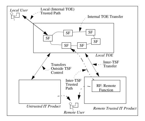
Figure 1.2 - Diagram of security functions in a distributed TOE
