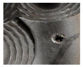
**Uneven Hardness Defect**
