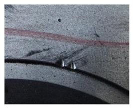
**Mechanical Damage Defect**
