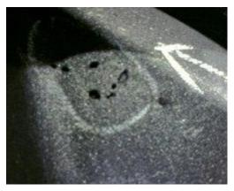
**Shrinkage Cavity Defect**
