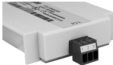
Figure 3: EIA-485 (RS485) Interface Pin Designation
