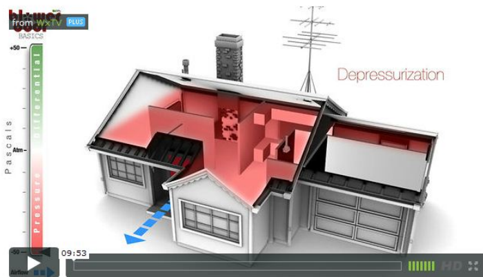
Figure 4. WxTV, Blower Door Basics: Part 3 – The Breakdown
