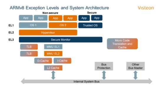
This architecture has three privileged exception levels. Exception level 1 is owned by the operating system and allows to configure the first level Memory Management Unit (MMU).
