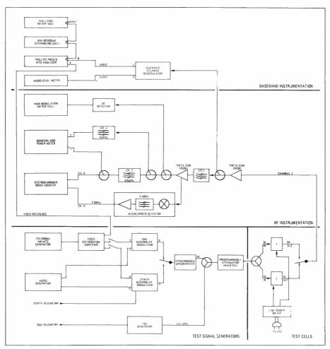
Figure 10 RF and video interconnection diagram
