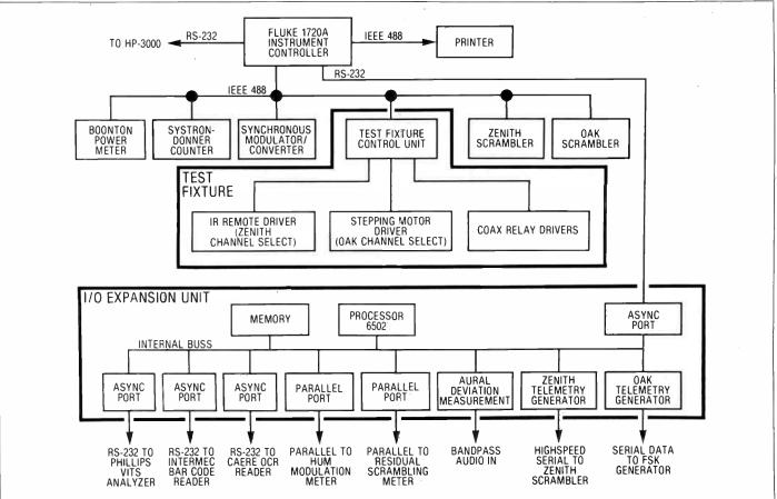
Figure 5 Control diagram-new test system
