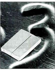
The cleaved coupled-cavity laser is a semiconductor laser cleaved into two nearly equal parts.
