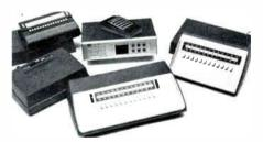
With Jerrold's outdoor descramblers, the descrambling electronics is in a rugged, weather-proof, RF-sealed housing for strand, eave or pedestal mounting—inaccessible to the subscriber. All indoor descramblers contain a self-destruct, anti-tamper device to prevent theft of services and equipment.
