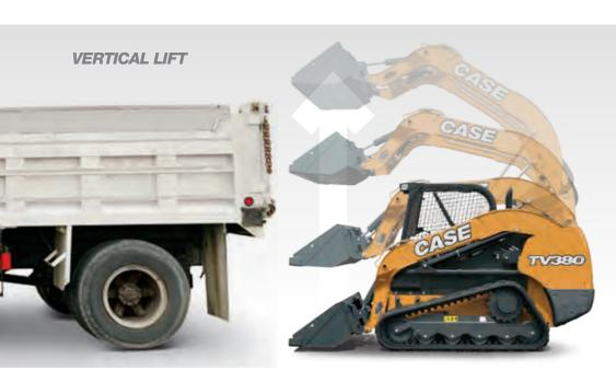
Vertical-lift machines are engineered for lift-and-carry and truck-loading jobs. The geometry of the dual arm allows the load to rise directly up, providing maximum reach at full height. Vertical-lift machines are ideal for reaching over the side of and into the middle of high-side trucks.
