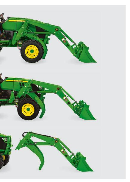
Quik-Park™ loader mounting system: R Series Loaders are designed for easy, tool-free mounting and removal. The parking stand is attached to the front frame of the tractor and becomes an integral part of the loader during loader operation. To drop the loader to the 'park' position, just lift the joystick after opening the latches.
