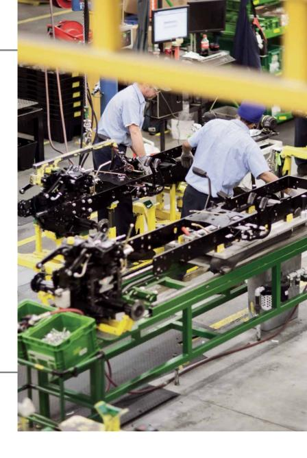
A transmission is being mounted onto the high-strength steel frame of a compact utility tractor by two Augusta factory workers.
