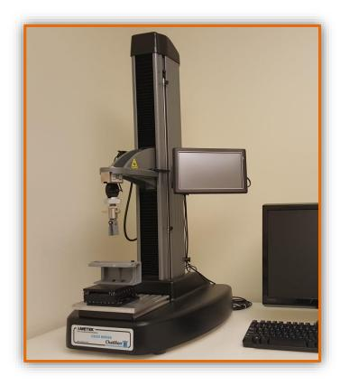
Mechanical force gage and test stand
