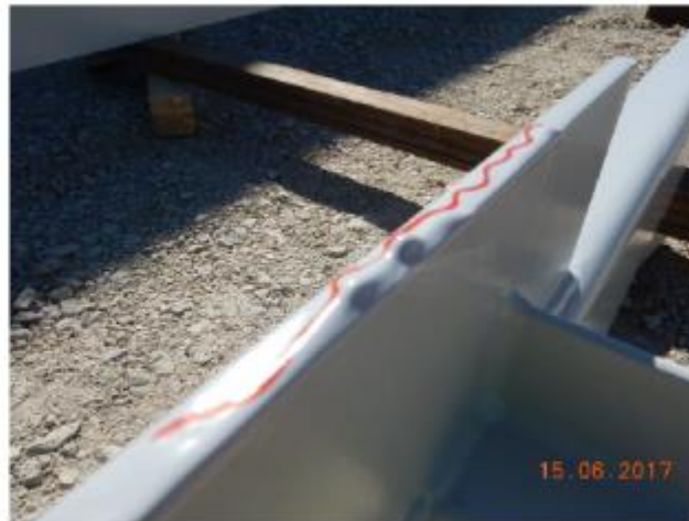
12. Paint defect (sagging)
