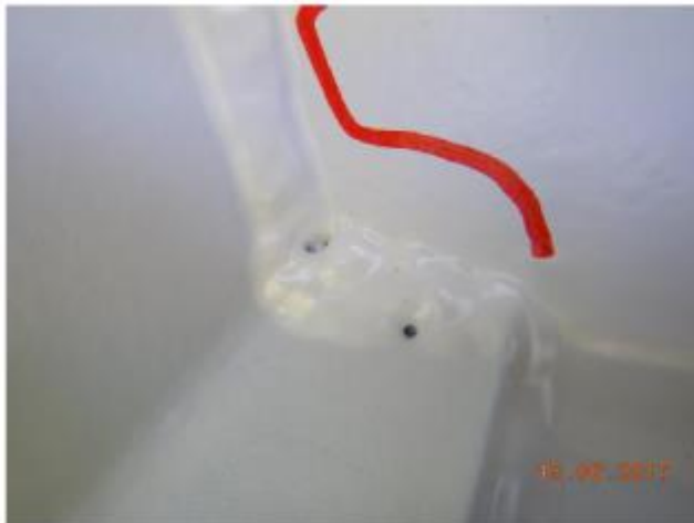
11. Weld defect (crater pipes, pores) with platforms
