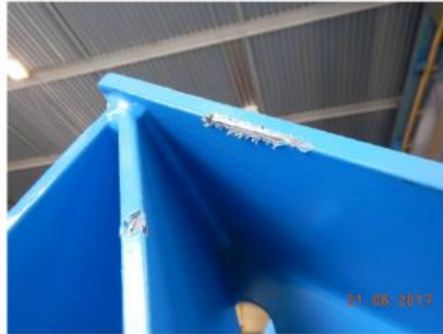
12. NC4: Paint damages with 1109 frame
