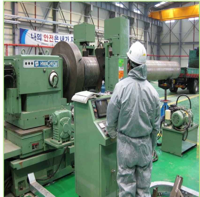
Beveling by End Facing CNC M/C
