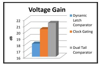
Fig6. Comparison Chart of Voltage Gain
