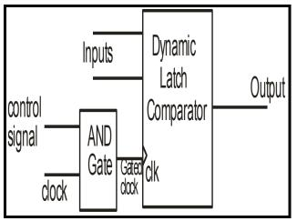
Fig3. Dynamic Latch Comparator using Clock Gating
