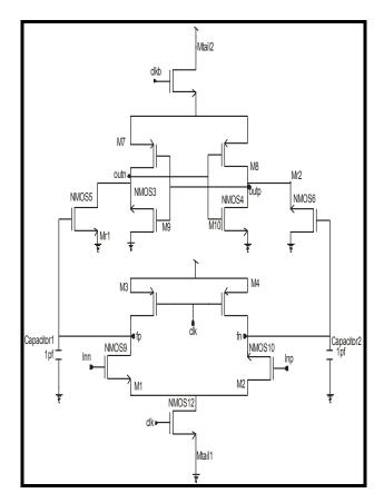
Fig4. Dual Tail Comparator Circuit
