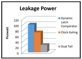
Fig8. Comparison Chart of Leakage Power
