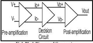
Fig1. Block Diagram of Comparator
