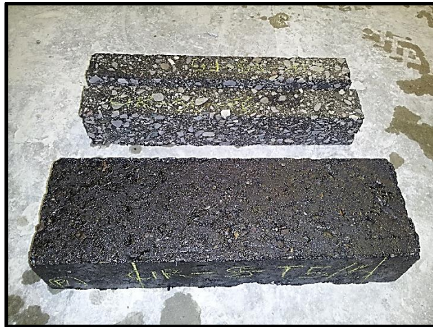
Figure 3-13: Mix sample beams cut out for testing
