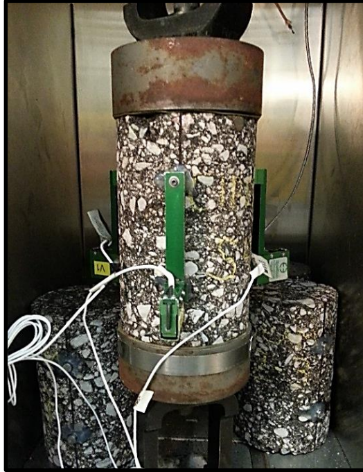
Figure 3-10: Dynamic modulus test setup in environmental chamber
