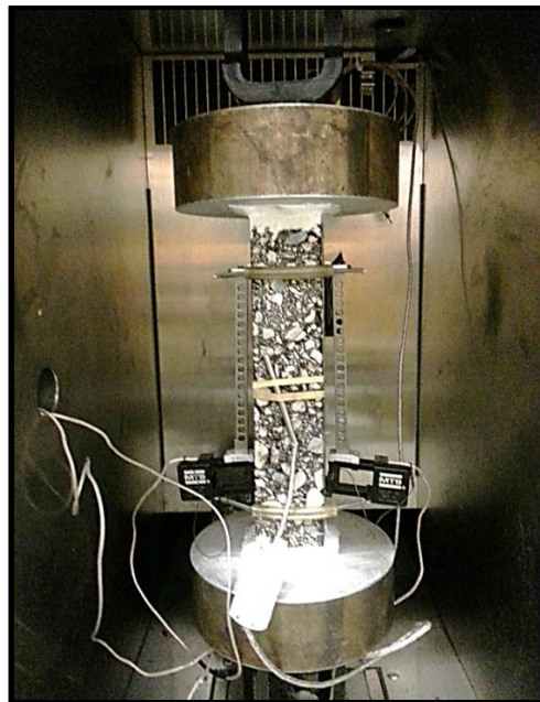
Figure 3-14: TSRST apparatus in an environmental chamber
