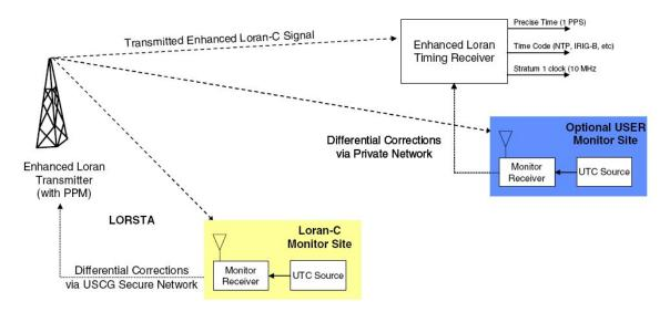
Figure 9. USCG monitoring sites provide the differential corrections included in eLORAN broadcasts.
