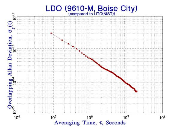
Figure 7. Frequency stability of LORAN 9610-M signals for averaging times ranging from one to 30 days.
