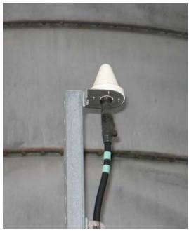
Figure 4. A GPS antenna at a CDMA base station with an obstructed view of the sky.
