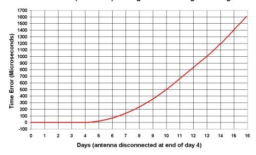
Figure 5. Phase plot of rubidium GPSDO with poor holdover capability during simulated signal outage.
