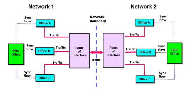
Figure 1. A plesiochronous connection between two networks. Each network maintains its own PRS.
