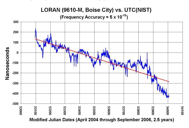
Figure 6. 30 month phase comparison between LORAN 9610-M and UTC(NIST).
