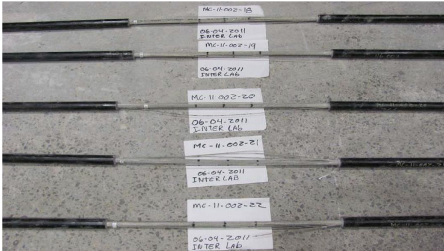
Figure 3. Failure of tensile specimens
