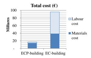
Figure 4: Material and labour cost of both buildings
