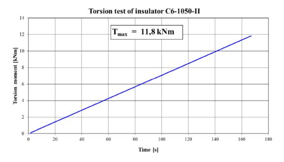
Graph. 5. Torsion Test with Isostatic Insulators.
