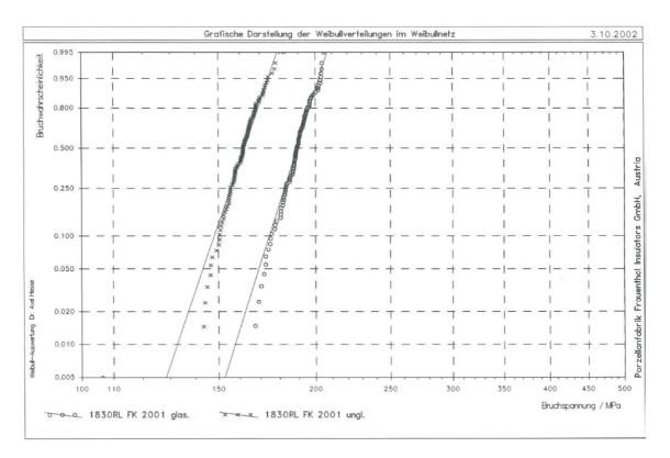
Graph. 2: 3-Point-Bending Test Weibull-Analyse of Plastic C 130 Porcelain
