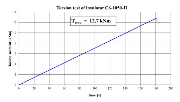
Graph. 6. Torsion Test with Plastic Insulator
