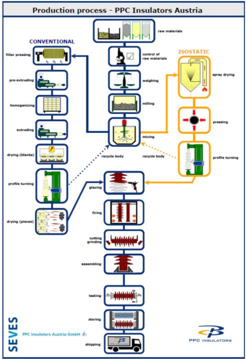
Fig. 1: The Plastic and Isostatic porcelain manufacturing process.
