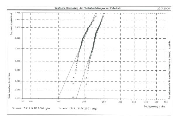
Graph. 1: 3-Point-Bending Test Weibull-Analyse of Isostatic C 130 Porcelain
