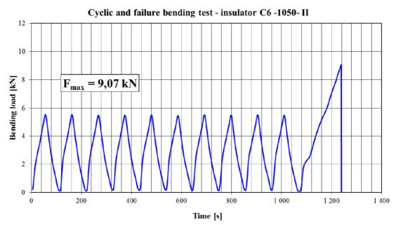
Graph. 4. Cyclic and Bending Failure Test with Plastic Insulators.
