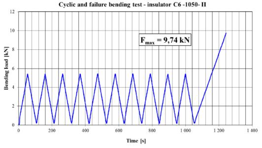
Graph. 3. Cyclic and Bending Failure Test with Isostatic insulators.
