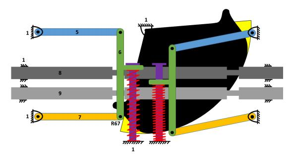
Figure 56 Unlocking and rotating discs at the locked position of the machine
