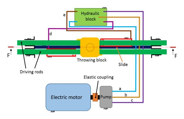
Figure 85 Schematic representation of installation of driving rods from top view
