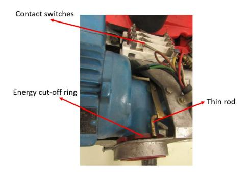
Figure 110 Energy cut-off mechanism
