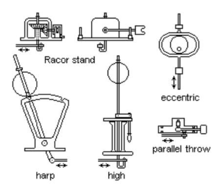
**Figure 5** Schematic views of different switch stand designs [3]
