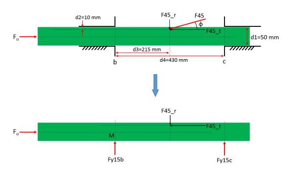
Figure 67 Free body diagram of link 5
