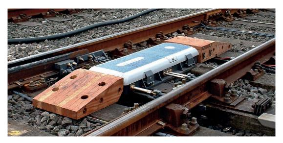
**Figure 16** Switchguard Surelock point machine mounted between the rails (the wooden wedges protect the machine from a derailed wheel) [14]
