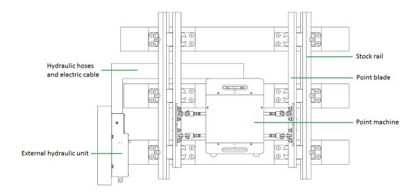
Figure 25 Schematic view of Easydrive-i installation [18]
