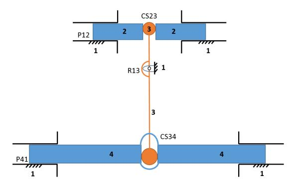
Figure 41 Kinematic joint types between the links
