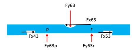
Figure 88 Free body diagram of shutter plate
