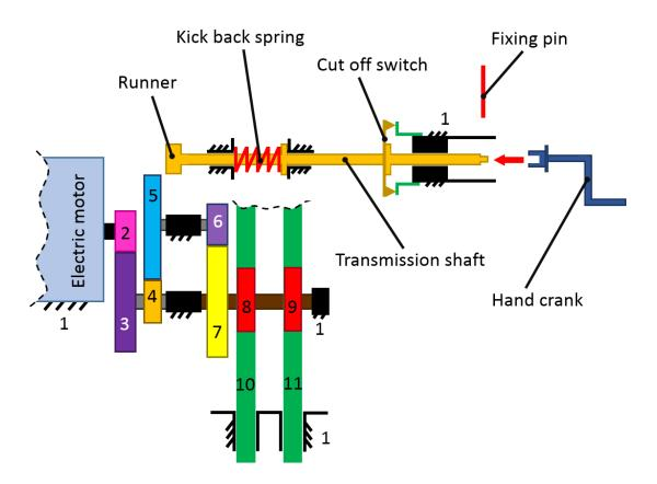
Figure 138 Schematic representation of manual operation assembly
