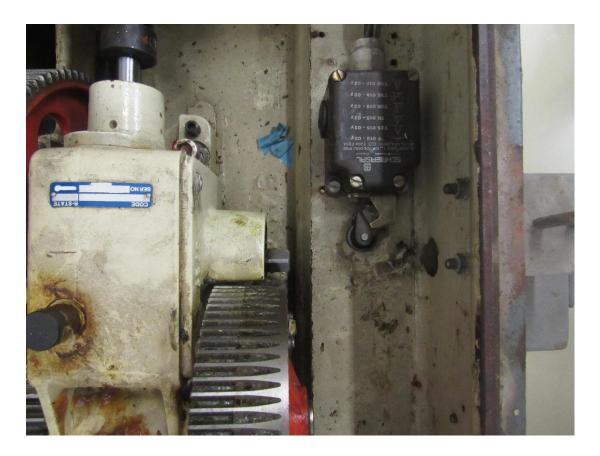
Figure 82 Safety cut out switch for manual operation
