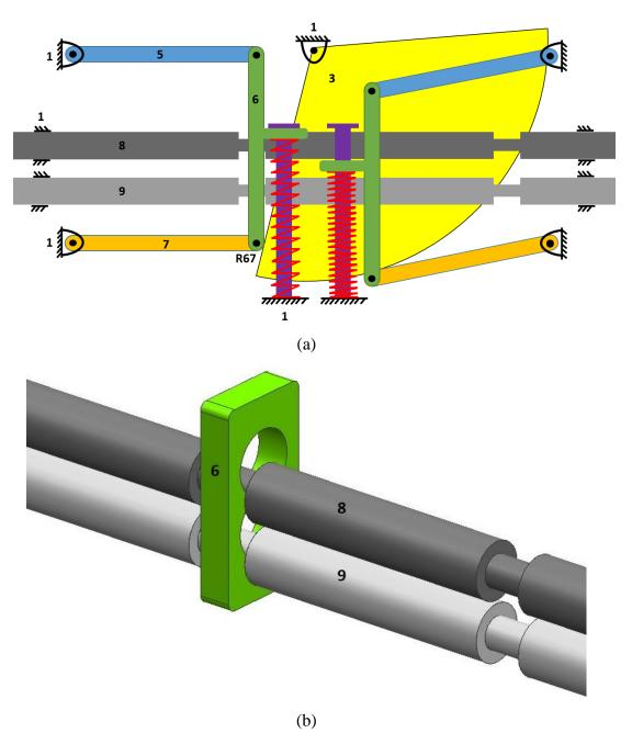
**Figure 53** Schematic representation of locked position of the machine (a) and the position of detector rods passing through the link 6 (b)
