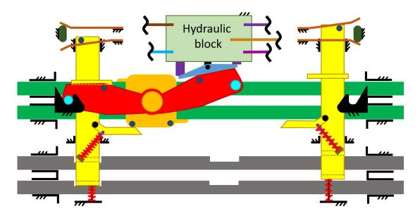
Figure 106 Locked position of the contact switches at the left hand side
