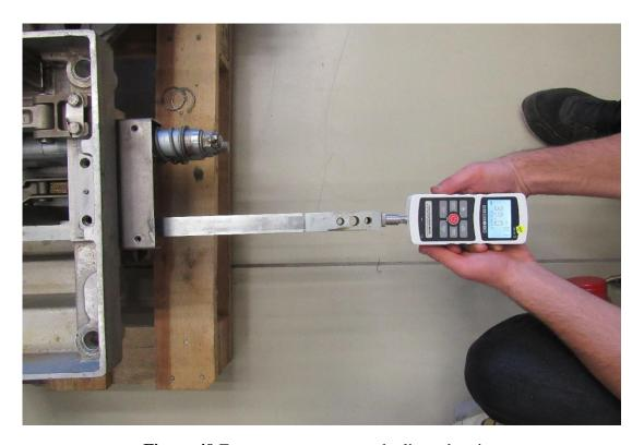
Figure 49 Force measurement at the linear bearing
