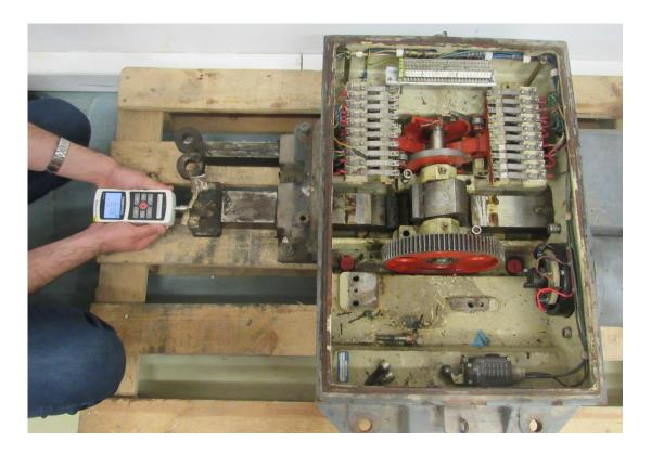
Figure 74 Force measurement at the linear slides
