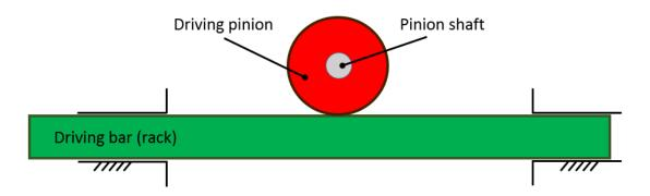
Figure 119 One of the rack and pinion gear mates from side view
