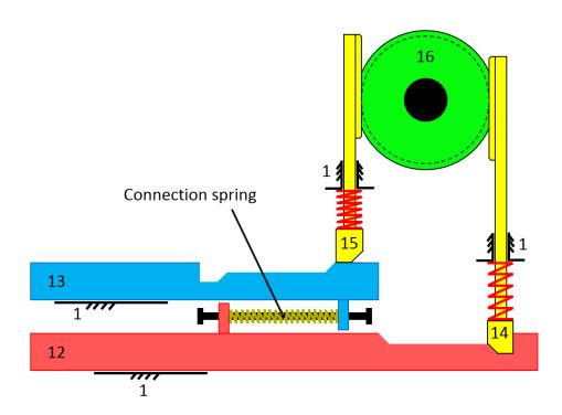
Figure 135 Schematic representation of locked position of the detection mechanism
