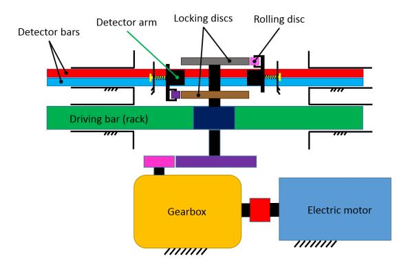
**Figure 76** Representative schematic model of locking mechanism together with the driving mechanism from top view
