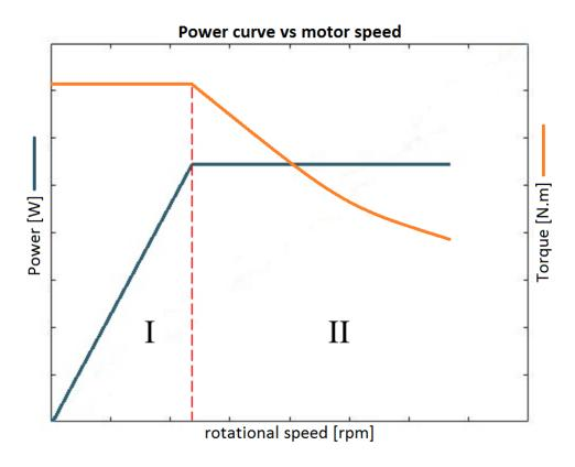
Figure 122 Typical power curve of a DC electric motor
