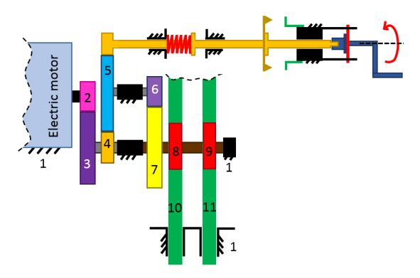
Figure 139 Schematic representation of use of hand crank
