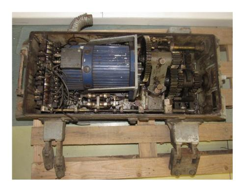
Figure 115 Photograph of inside view of point machine D
