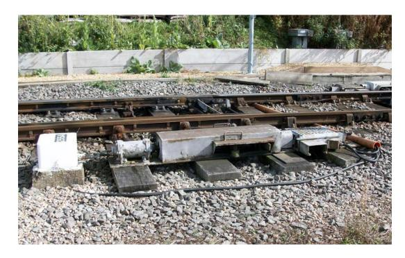
**Figure 10** An electro-pneumatic point machine fitted to 225A points, north of Bletchey Station in England, 27.09.2012. [10]
