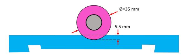
Figure 113 Mating of trailing cylinder into shutter plate seat
