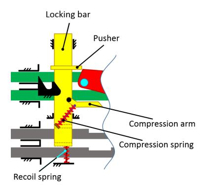
Figure 99 Schematic representation of locking mechanism for detector rods
