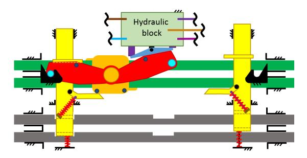
Figure 102 Locked position of the machine at the left position
