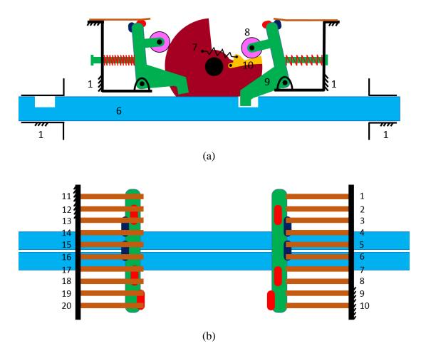
**Figure 81** Position of the contact switches from front (a) and top (b) views for one of the locked positions
