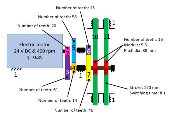
Figure 118 Known and measured parameters of the driving mechanism
