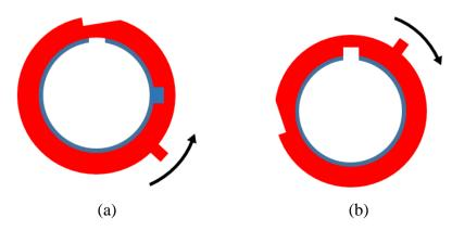
**Figure 109** Position of the energy cut-off ring in normal (a) and manual (b) operations
