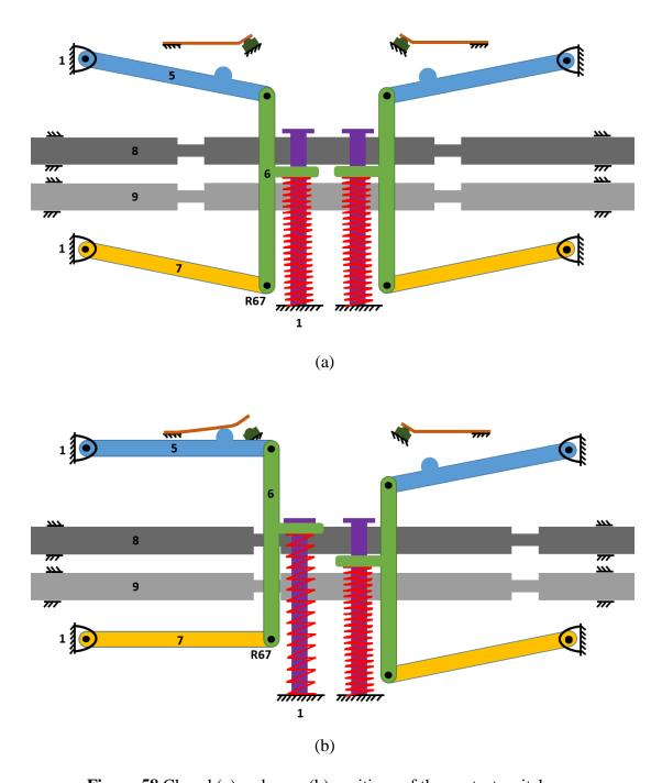
Figure 58 Closed (a) and open (b) positions of the contact switches
