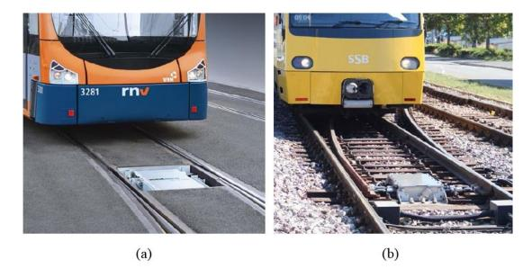
**Figure 20** Unistar CSV 24 point machine embedded track, 1000 mm track gauge (a) and open track, 1435 mm track gauge (b) [16]
