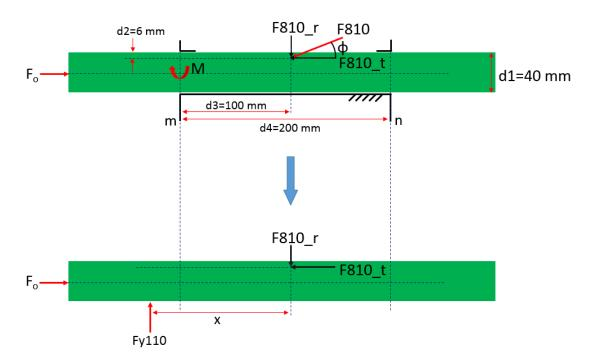
**Figure 121** Free body diagram of component 10
