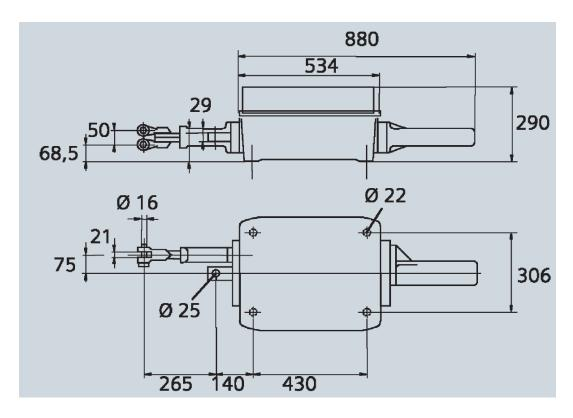
Figure 14 Some important dimensions of S 700 K in mm [13]
