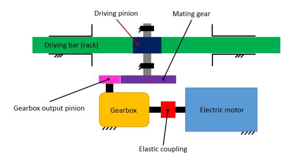
Figure 61 Representative schematic model of driving mechanism from top view
