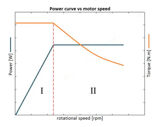
Figure 68 Typical power and torque curve of a DC electric motor
