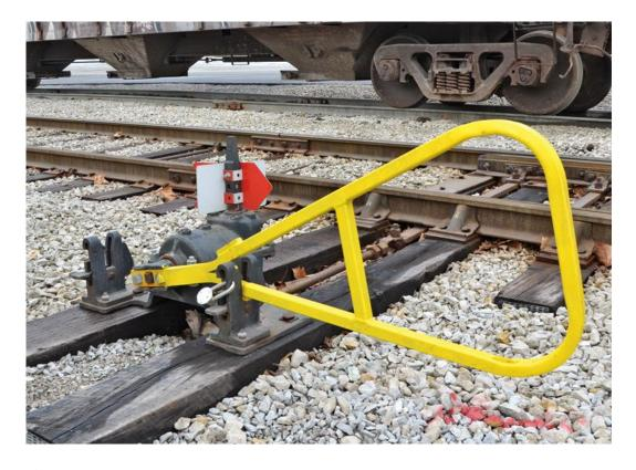
Figure 7 An example of racor type point lever and padlocked latch in a position [5]
