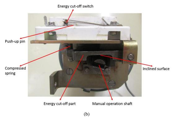
Figure 59 Three energy cut-off switches (a) and energy cut-off mechanism (b)
