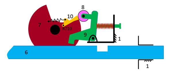
Figure 79 Schematic representation of locking delay
