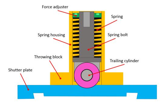
Figure 111 Components of retaining assembly
