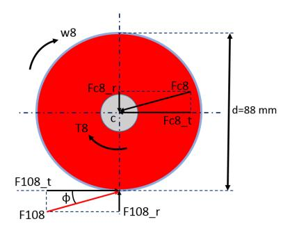
Figure 120 Free body diagram of the gear 8
