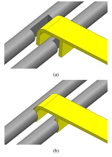
Figure 103 Unlocked (a) and locked (b) positions of the detector rods
