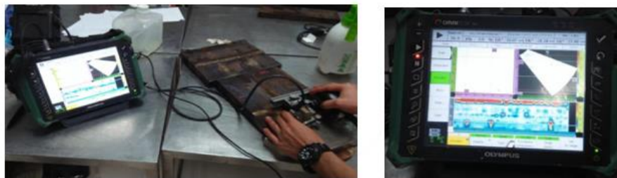
Figure 8: Detection and measuring planar defects height in test plates using PAUT.
