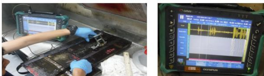
Figure 9: Detection and measuring planar defects in test plates using TOFD.
