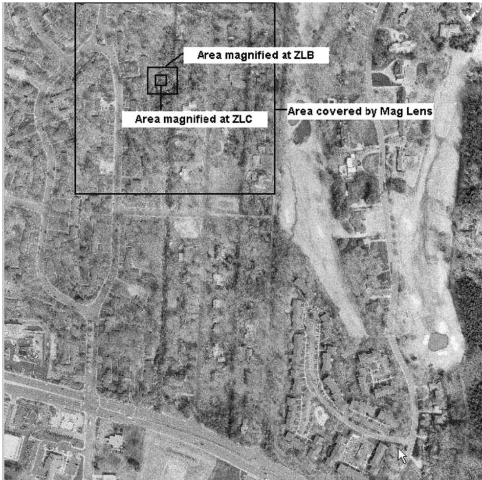
Fig. 2. MagLens magnification area vs area covered by the lens. ZLB is ZL3 and ZLC is ZL4 for the MagLens interaction method.
