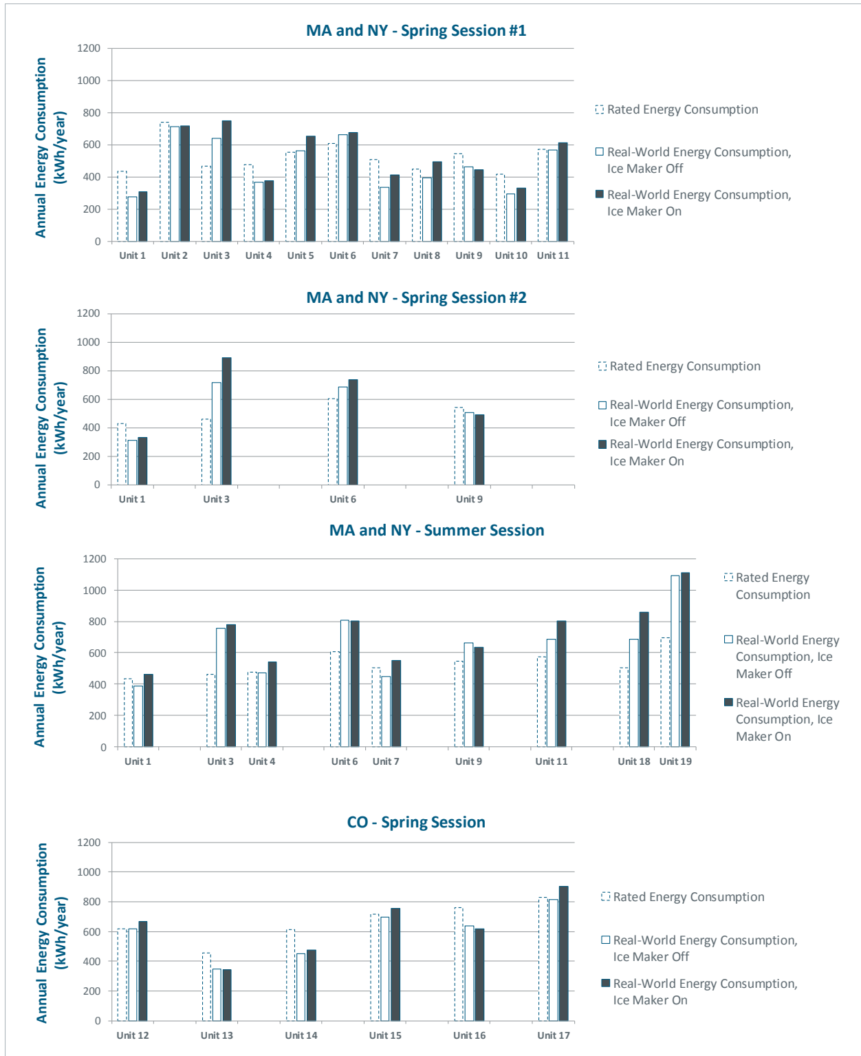
Figure 2. Comparison of rated energy consumption, energy consumption with ice maker off, and energy consumption with ice maker on
