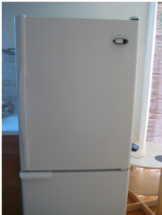
Figure 27. Installation of USB Track-It Data Logger
