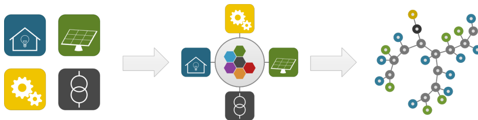
Figure 5.1: Schematic of a typical Mosaik use case [30]. Blue represents household simulators, green PV simulators, gray a load flow analysis tool, and yellow a monitoring and analysis tool [30]. A coordinated simulation can be started after the four simulators were connected to Mosaik. A visualization of the simulation can be seen in the last step of the schematic which uses the same color scheme as before.
