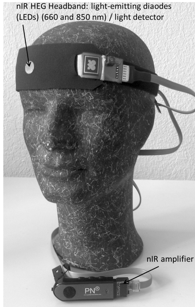
Figure 2. Wireless fNIRS instrument (Biocomp Research Institute, nIR system). The single-distance continuous-wave spectroscopy instrument consists of one channel with one light source with light-emitting diodes (LEDs) (two different wavelengths at 660 nm and 850 nm) and one light detector with a source-detector distance of 3 cm and a size 90 x 40 mm. The centre of the sensor was positioned covering F8 according to the international 10-20 system (Jaspers, 1958).
