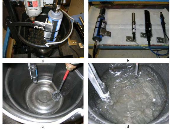
**Figure 4.** Sediment mixing apparatus. (a) Mixing bucket, drill and sensor stand, (b) sensors and mounting brackets, (c) locations of mixing paddle and sensor, (d) measuring in the mixed sediment suspension.
