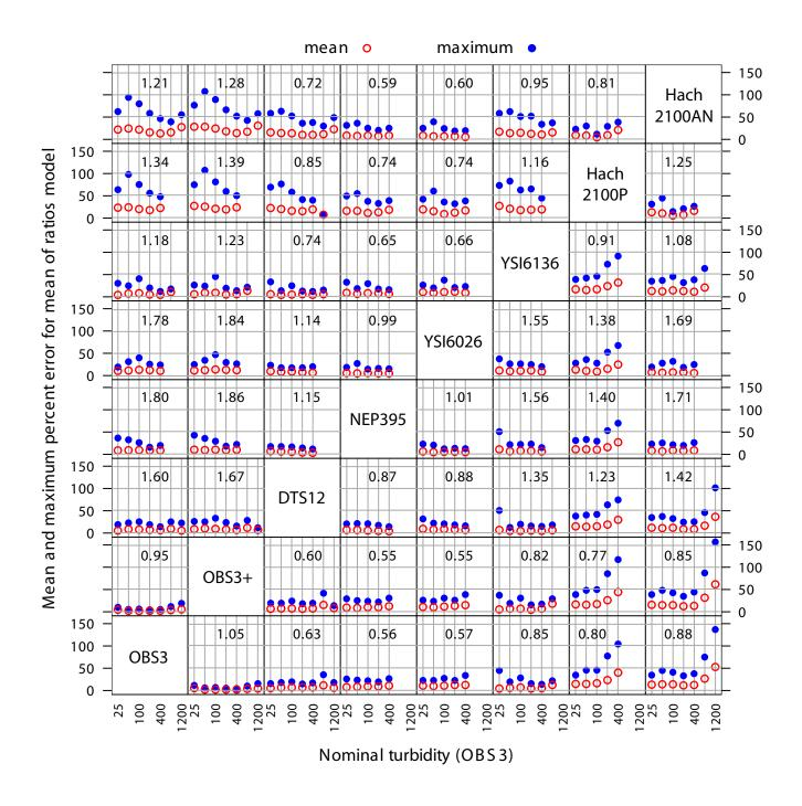
Figure 11. Mean and maximum errors for ratio model relating all pairs of sensors. The number displayed in each graph is the estimated ratio, based on the mean of ratios model. For each graph, the predictor is the sensor whose name is on the diagonal in the same column and predicted value is for the sensor whose name is on the diagonal in the same row.
