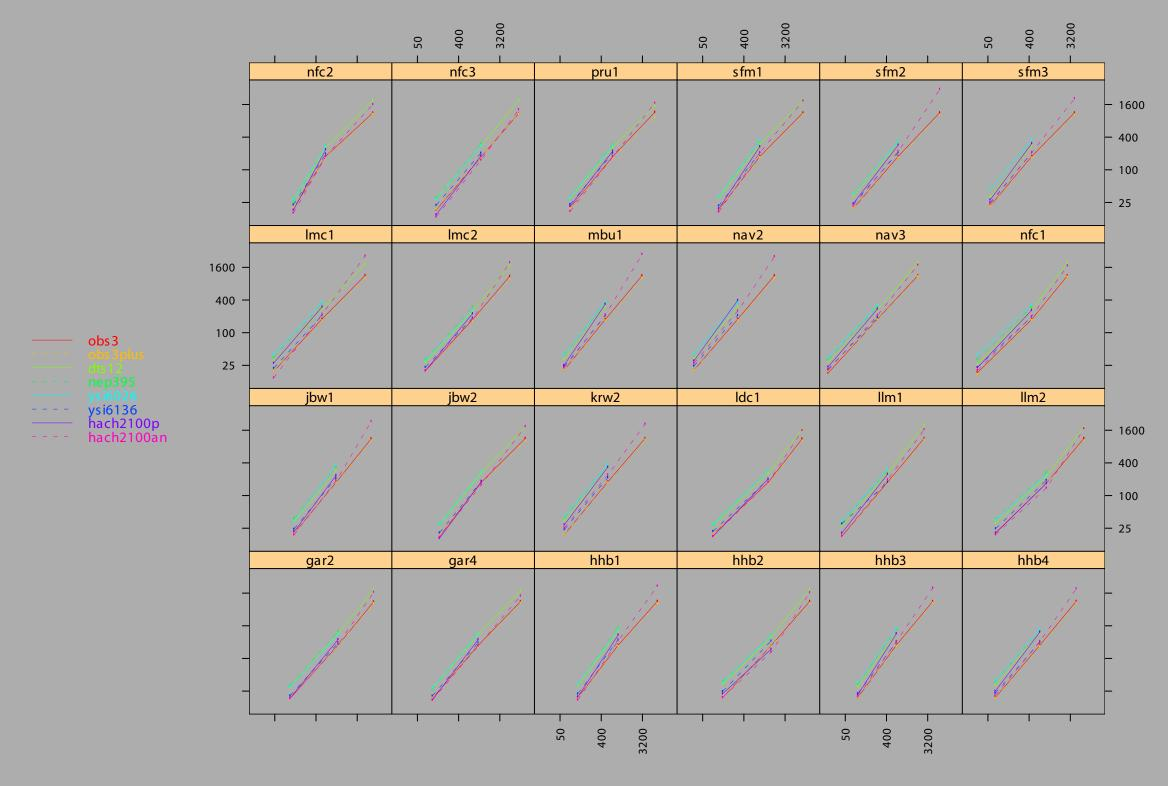
Figure 8. Turbidity is plotted as a function of SSC for each sensor by sediment. Each sediment was sampled at nominal turbidity levels of 25, 200, and 1200 units as measured by the OBS-3 sensor. The YSI 6026, YSI 6136, NEP395, Hach 2100P, and some of the DTS-12 readings are off-scale at the 1200 level and are not shown.
