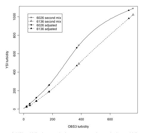
**Figure 6.** YSI turbidity in second mix was converted to equivalent turbidity in first mix (shown as "adjusted" in legend) by interpolation from the relation between YSI and OBS-3 turbidities, illustrated for sample LMC2.
