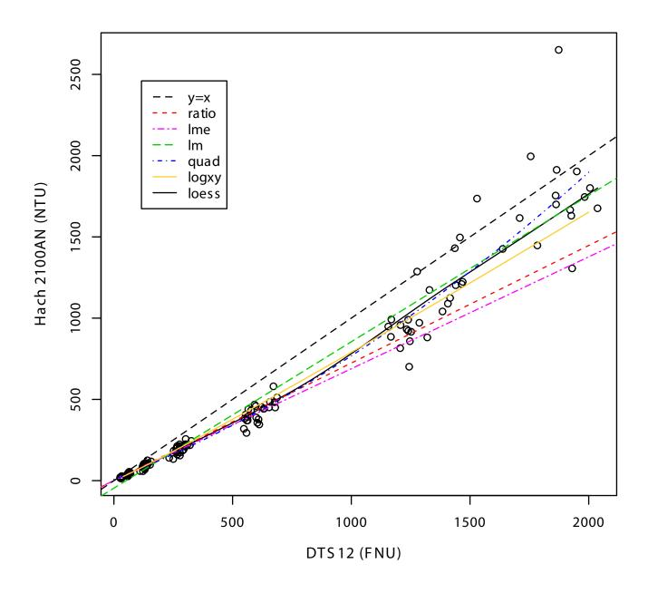
Figure 12. Six models for converting DTS-12 data to Hach 2100AN. Data for nominal turbidity levels from 25 to 1200 are included for all 24 sediment types.
