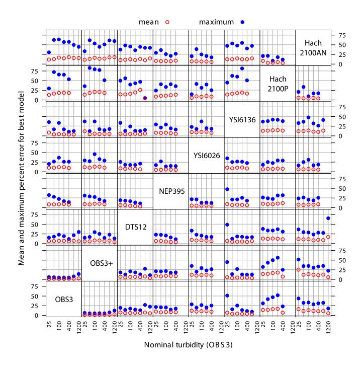
Figure 13. Mean and maximum errors for the best model (see Table 6) relating each pair of sensors. For each graph, the predictor is the sensor whose name appears on the diagonal in the same column and the predicted turbidity is for the sensor whose name appears on the diagonal in the same row.
