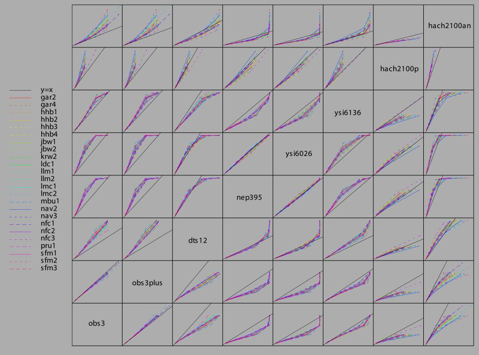
Figure 9. Scatterplot matrix, showing the relationships among turbidity readings for all pairs of sensors. Each line represents one sediment type. Out-of-range data have *not* been omitted, except for the Hach 2100P. The x variable for a given plot is the sensor whose name appears on the diagonal in the same row. The x and y scales are set by the range of data for the sensors in the corresponding column and row.
