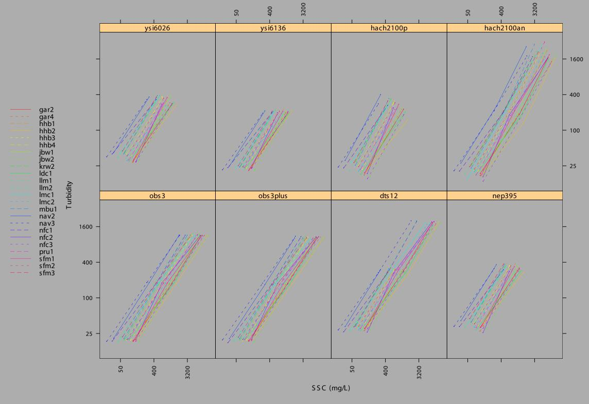
Figure 7. Turbidity is plotted as a function of SSC for each sediment by sensor. Each sediment was sampled at nominal turbidity levels of 25, 200, and 1200 units as measured by the OBS-3 sensor. The YSI 6026, YSI 6136, NEP395, Hach 2100P, and some of the DTS-12 readings are off-scale at the 1200 level and are not shown.
