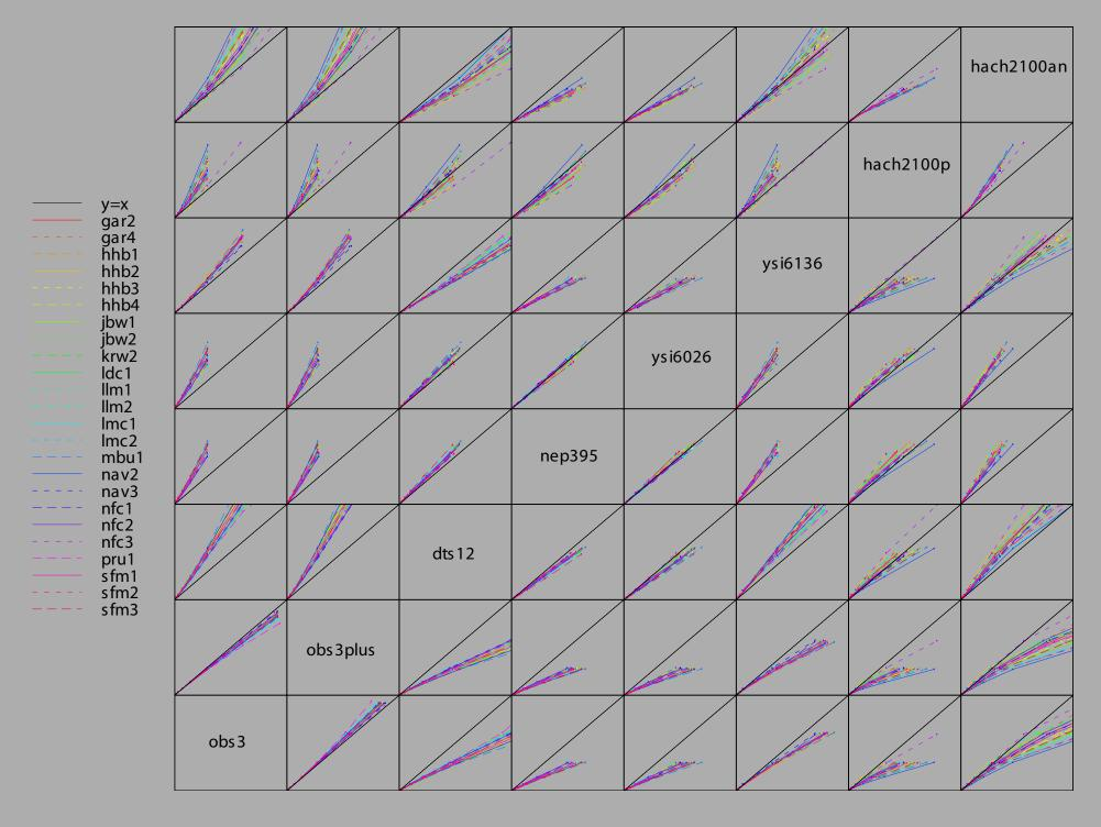
Figure 10. Scatterplot matrix, showing the relationships among turbidity readings for all pairs of sensors. This figure is similar to Figure 9 except that out-of-range data have been omitted and the ranges of all x and y scales are fixed at 0 to 1250. As a result, 29 DTS-12 points and 28 Hach 2100AN points above 1250 are not displayed.
