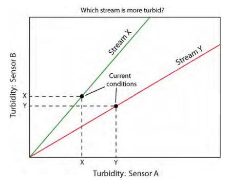
**Figure 1**. If relationships between sensors depend strongly on the stream being measured, then turbidity rankings of streams may differ by sensor.
