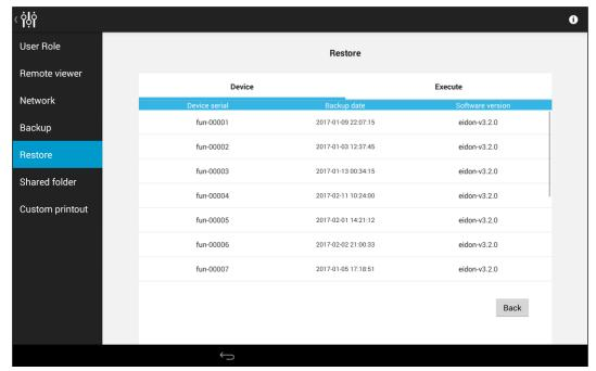
Fig. 70 - Configurator - RESTORE screen - List of available archives to be restored
