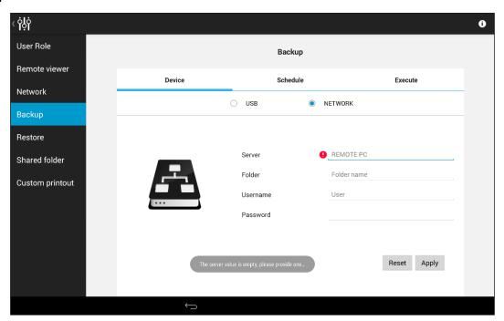
Fig. 66 - Configurator - BACKUP screen - Network backup selected
