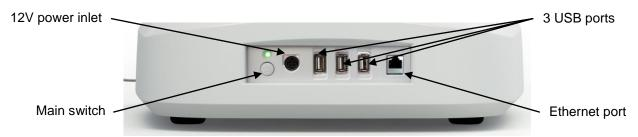
Fig. 2 – Detail of connectors side
