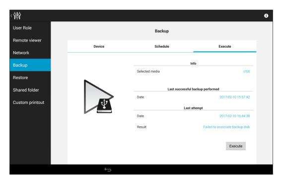
Fig. 68 - Configurator - BACKUP screen - Execute tab
