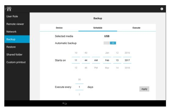
Fig. 67 - Configurator - BACKUP screen - Schedule tab with automatic backup enabled
