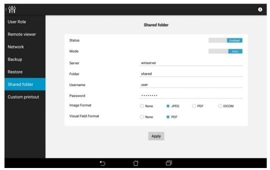
Fig. 71 – Configurator – SHARED FOLDER configuration
