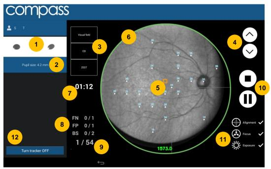
Fig. 28 – Exam screen while test is in progress
