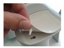
Fig. 73 - Removal of the chin rest silicon pad
