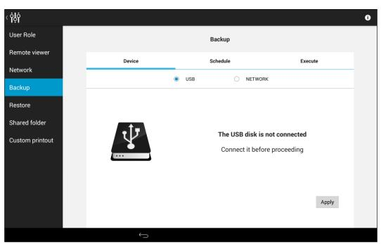
Fig. 65 - Configurator - BACKUP screen - USB-media backup selected
