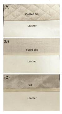
Fig. 1— Leather combined with silk based samples (A – leather with quilted silk, B – leather with fused silk, and C – leather with silk)
