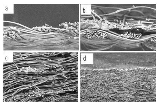
Fig. 3 — Scanning electron micrographs showing cross sectional view of silk based samples and leather (a) mulberry silk, (b) mulberry silk fused with non-woven fusing material, (c) mulberry silk quilted with foam and (d) leather
