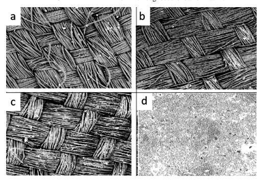
Fig. 2 — Scanning electron micrographs showing surface fibre pattern of silk based samples and leather (a) mulberry silk, (b) mulberry silk fused with non-woven fusing material, (c) mulberry silk quilted with foam and (d) leather
