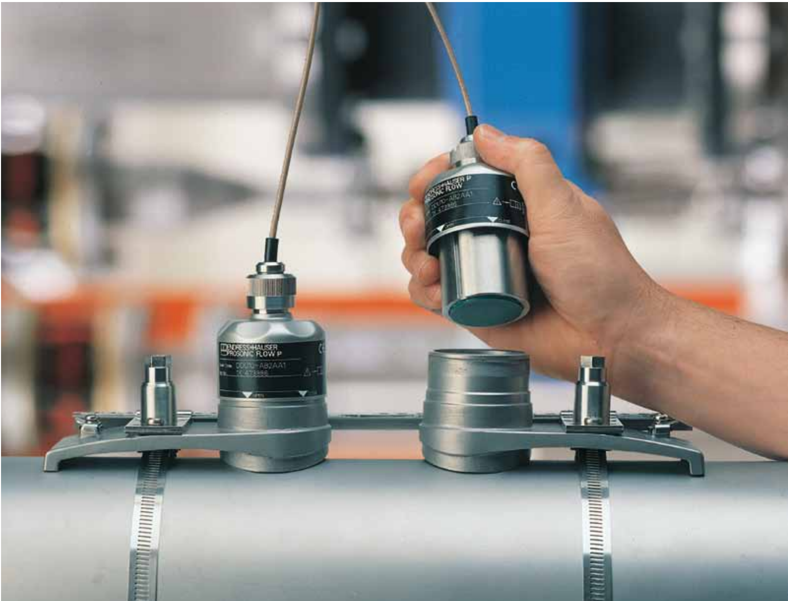
Clamp on ultrasonic flow measurement in the main pipe. CFE CH La Boquilla, Chihuahua México
