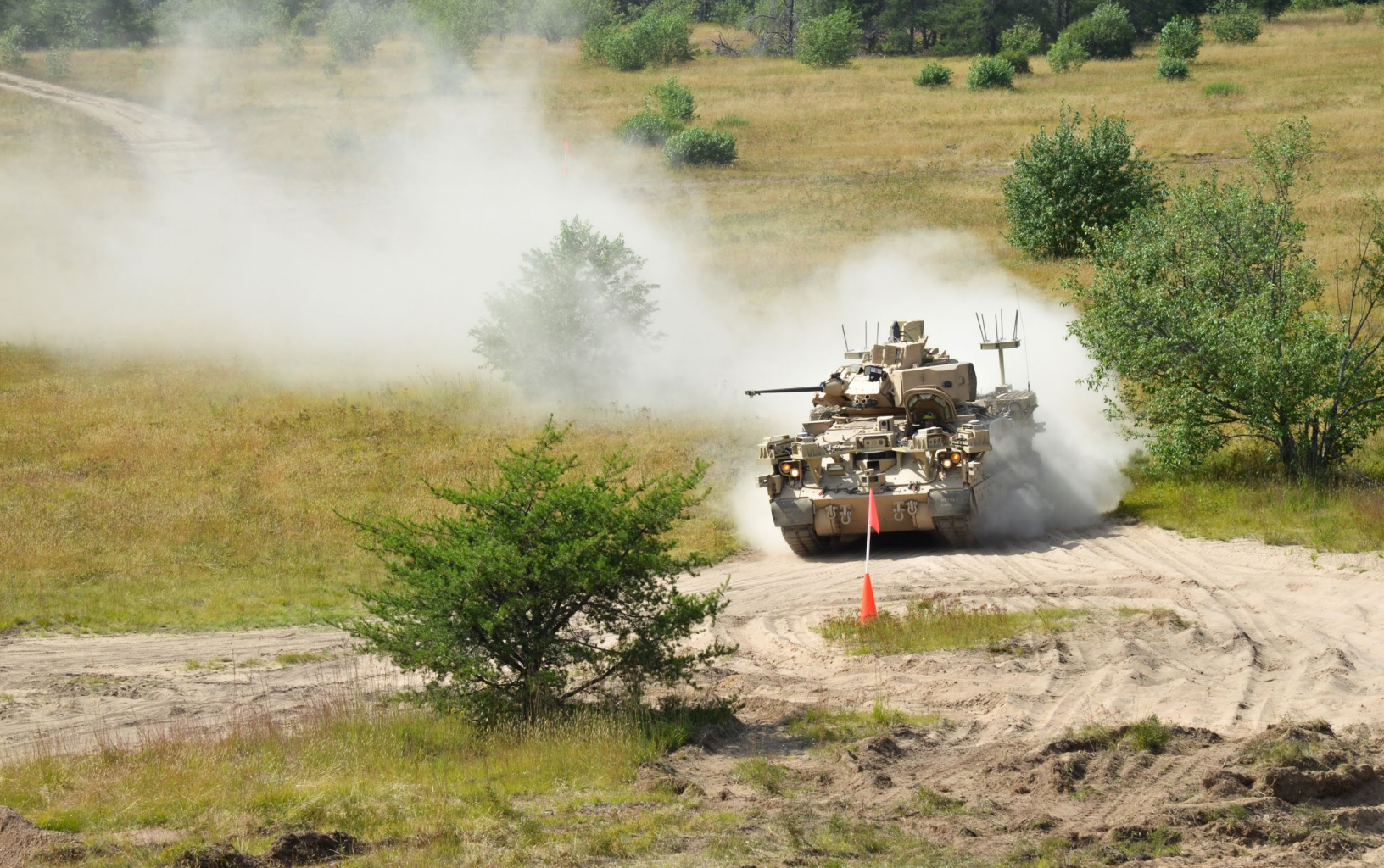
Army Modernization Priority 2: Next-Generation Combat Vehicles (NGCVs) to increase the firepower, speed, maneuverability, and survivability of land forces. Here, this Mission Enabling Technologies Demonstrator (MET-D) manned vehicle can operate two unmanned ground platforms to make contact with the enemy before soldiers do. Source: US Army photo by Jerome Aliotta https://www.army.mil/article/226774/army_demos_prototype_manned_fighting_vehicle teamed_with_robotic_combat_vehicle_platoon
