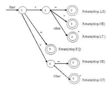
As an intermediate step in the construction of a LA, we first produce a stylized flowchart, called a transition diagram. Position in a transition diagram, are drawn as circles and are called as states.
