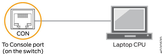
Figure 54: Connecting a Switch Directly to a Management Console
