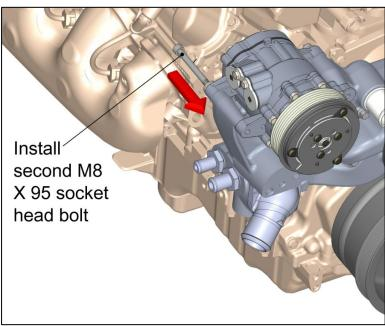
**NOTE:** After assembly torque M8 bolts to 18 ft./lbs.
