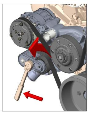
After routing the belt use a 1/2" square drive wrench to pull the tensioner all the way down and work the belt on from the rear.
