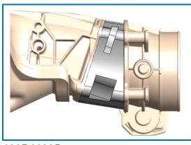
Throttle Body Angle Correcting Adapter (LT applications only):
