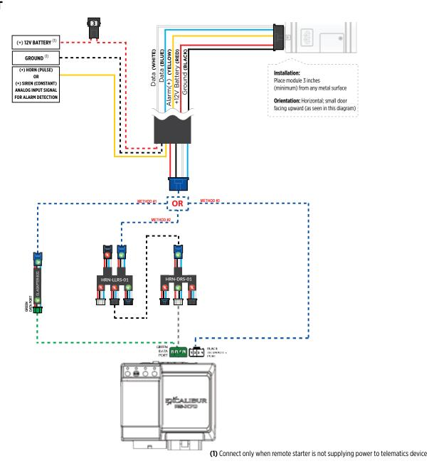
Once the telematics module is connected into the remote starter, two LED's will display to which networks you are connected to. (See LED Status Reference Chart on last page for details). **NOTE: The vehicle may need to be outside in an open area in order to connect to a cellular and/or GPS network.**
