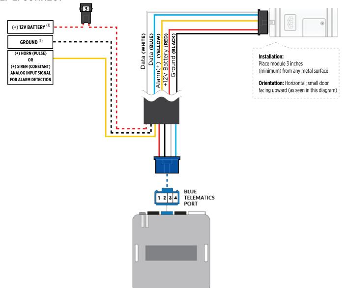
Once the telematics module is connected into the remote starter, two LED's will display to which networks you are connected to. (See LED Status Reference Chart on last page for details). **NOTE: The vehicle may need to be outside in an open area in order to connect to a cellular and/or GPS network.**
