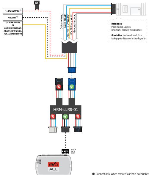
Once the telematics module is connected into the remote starter, two LED's will display to which networks you are connected to. (See LED Status Reference Chart on last page for details). **NOTE: The vehicle may need to be outside in an open area in order to connect to a cellular and/or GPS network.**
