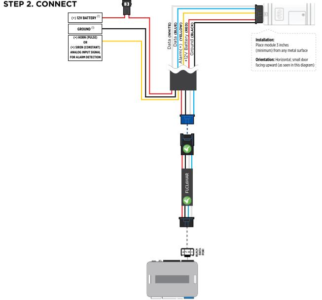
Once the telematics module is connected into the remote starter, two LED's will display to which networks you are connected to. (See LED Status Reference Chart on last page for details). **NOTE: The vehicle may need to be outside in an open area in order to connect to a cellular and/or GPS network.**
