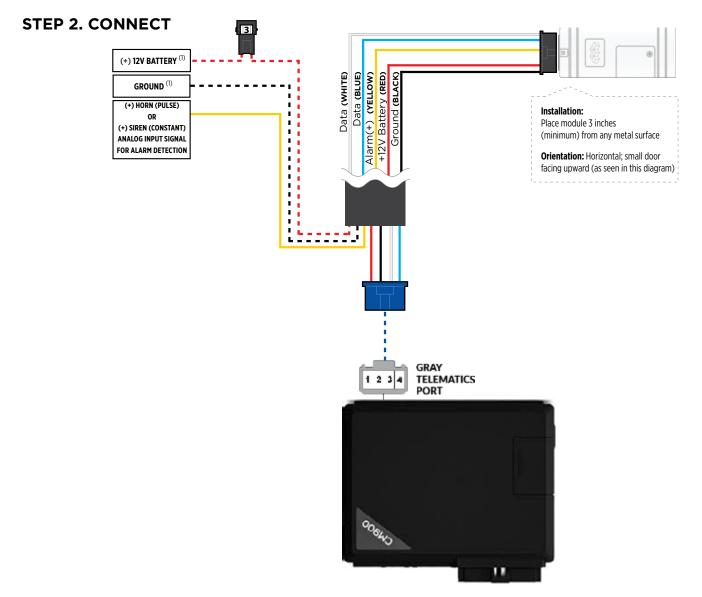
Once the telematics module is connected into the remote starter, two LED's will display to which networks you are connected to. (See LED Status Reference Chart on last page for details). **NOTE: The vehicle may need to be outside in an open area in order to connect to a cellular and/or GPS network.**
