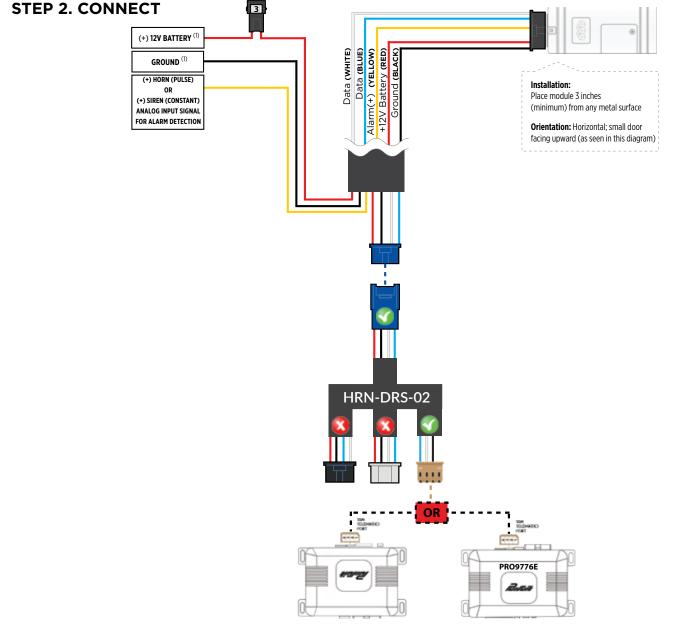
(1) Connect to supply power to telematics device
