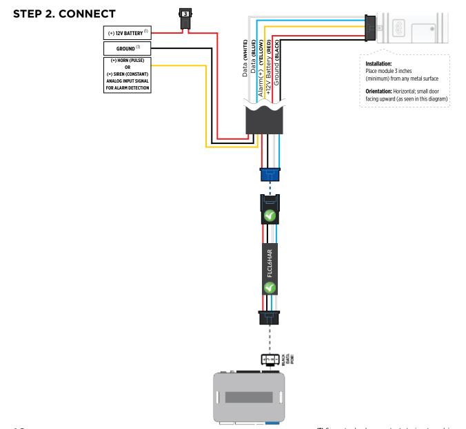
Once the telematics module is connected into the remote starter, two LED's will display to which networks you are connected to. (See LED Status Reference Chart on last page for details). **NOTE: The vehicle may need to be outside in an open area in order to connect to a cellular and/or GPS network.**
